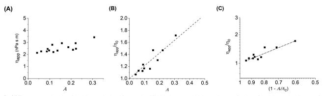
Fig. 5 (A) The apparent viscosity of the bilayer calculated from probe diffusivity increases with increasing area fraction of particles on the bilayer surface. (B) The apparent viscosity scaled by the dilute viscosity, showing a linear increase. (C) The same data plotted against the critical area fraction in analogy to 2D monolayer and 3D suspensions to test a power law behavior.
