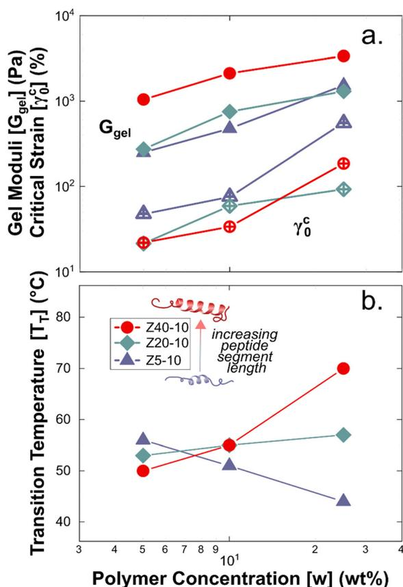
Fig. 5 Summary of the rheology of PPU hydrogels as a function of concentration and peptide segment length. (a)  $G_{\text{gel}}$  (filled symbols) and  $\gamma_0^c$  (open symbols). (b) Transition temperature measured under increasing temperature at a frequency of  $100 \text{ rad s}^{-1}$ .
