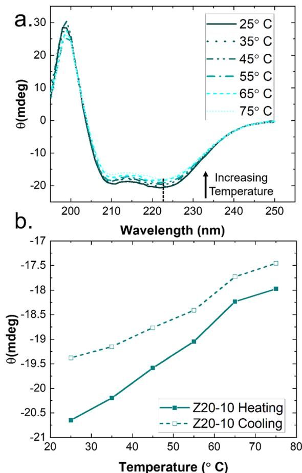
Fig. 7 Temperature modulated CD spectra of Z20-10. (a) Full wavelength scan shows  $\alpha$ -helical secondary structure is maintained over the entire temperature range; only very slight melting can be observed. (b) Monitoring the peak intensity at 222 nm reveals hysteresis in secondary structure recovery in a heating/cooling cycle. Points are taken from the temperature scans shown in (a).
