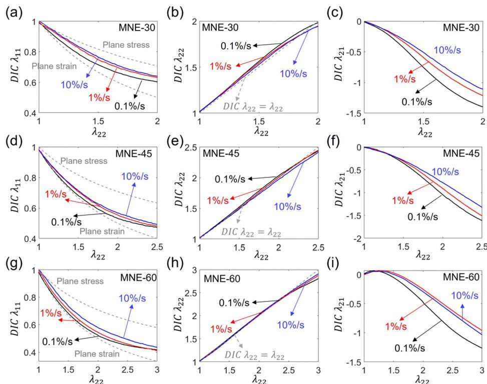
Fig. 6 Components of the deformation gradient,  $\lambda_{11}$ ,  $\lambda_{22}$ , and  $\lambda_{21}$ , measured by the DIC method as functions of the applied external stretch  $\lambda_{22}$  at different loading rates of 10%/s, 1%/s, and 0.1%/s for specimens (a), (d) and (g) MNE-30, (b), (e) and (h) MNE-45, and (c), (f) and (i) MNE-60, respectively.
