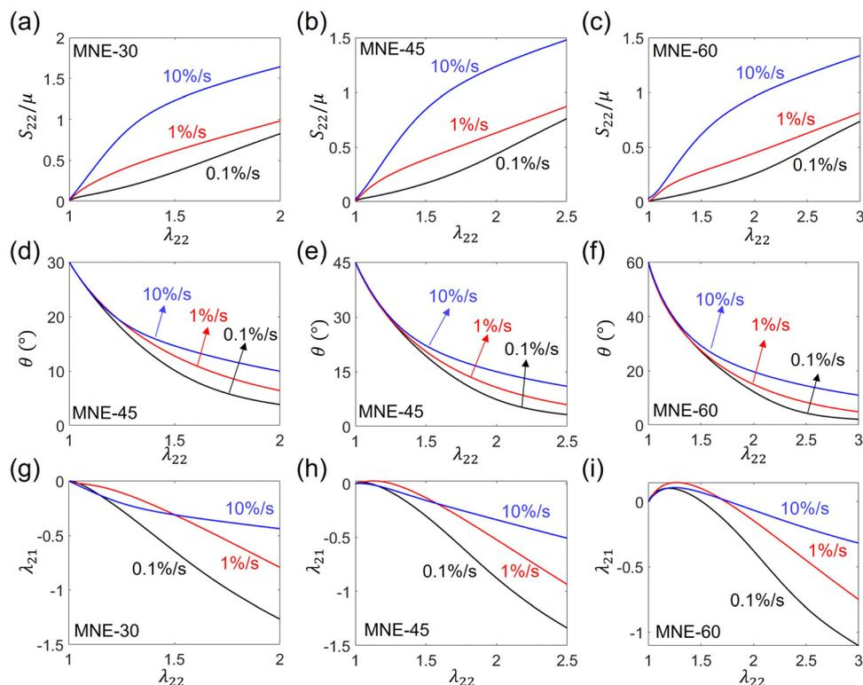
Fig. 10 Analytical results of the (a)–(c) engineering stress  $S_{22}$ , (d)–(f) director angle  $\theta$ , and (g)–(i) shear strain  $\lambda_{21}$  as functions of the normal stretch  $\lambda_{22}$  at different loading rates of  $10\%/s$ ,  $1\%/s$ , and  $0.1\%/s$  for MNE-30, MNE-45, and MNE-60, respectively.
