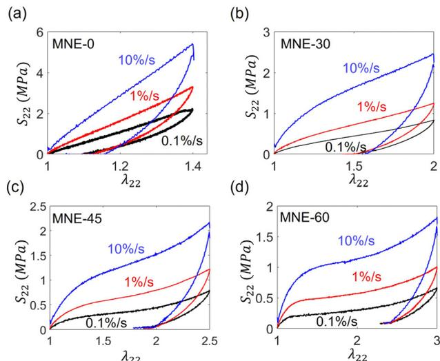
Fig. 4 Loading and unloading nominal stress ( $S_{22}$ ) as a function of the applied external stretch ( $\lambda_{22}$ ) for specimens (a) MNE-0, (b) MNE-30, (c) MNE-45, and (d) MNE-60 under uniaxial tension at loading and unloading rates of 10%/s, 1%/s, and 0.1%/s.
