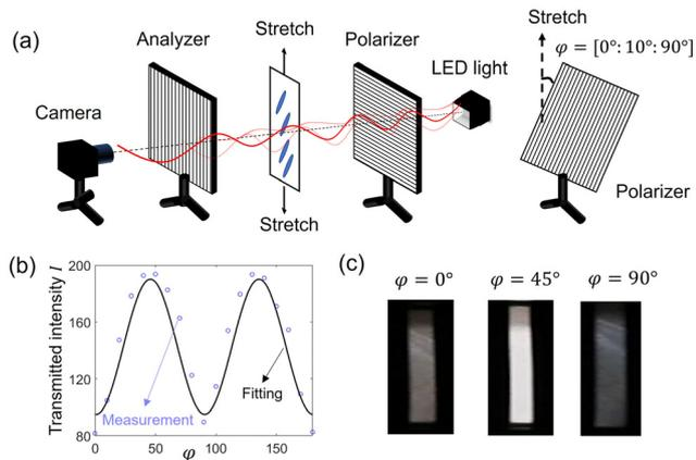
Fig. 2 (a) Schematics of the setup of the crossed-polarized optical measurement for directors. (b) The transmitted intensity  $I$  was measured as a function of the angle between the polarizer and the tension direction,  $\varphi$ , and fitted by eqn (1) to determine the director  $\theta$ . (c) The appearance of an MNE-0 specimen showing different brightness was captured by a camera with different angles  $\varphi = 0^\circ, 45^\circ$ , and  $90^\circ$ .
