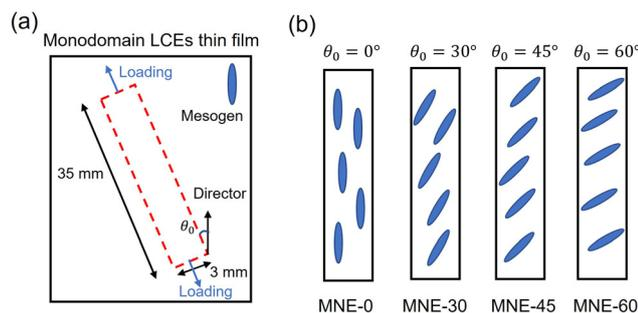
**Fig. 1** Schematics of specimens with different initial directors. (a) The specimen (red dashed line) was cut from a LCE thin film with the angle between the director and the longitudinal direction defined as  $\theta_0$ . (b) Specimens with different initial directors are defined as MNE-0, MNE-30, MNE-45, and MNE-60, corresponding to  $\theta_0 = 0^\circ, 30^\circ, 45^\circ$  and  $60^\circ$ , respectively. The specimens were 3 mm in width and 35 mm in length.
