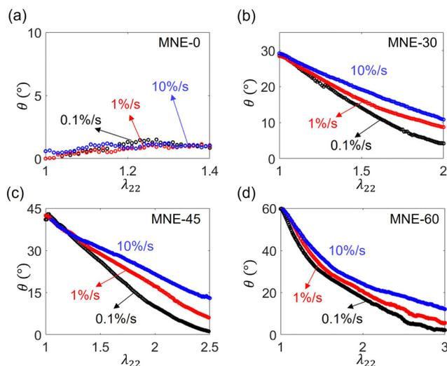
Fig. 5 Director reorientation as a function of the applied external stretch  $\lambda_{22}$  at loading rates 10%/s, 1%/s, and 0.1%/s for (a) MNE-0, (b) MNE-30, (c) MNE-45, and (d) MNE-60, respectively.
