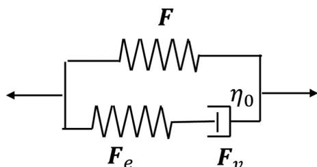
Fig. 9 Rheological model for the viscoelasticity of LCEs.
