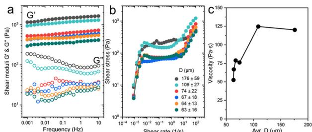
Fig. 2 Rheological characterization of jammed PAAm microgel suspensions. (a) Small amplitude oscillatory frequency sweeps that determine  $G'$  (solid circles) and  $G''$  (hollow circles). (b) Shear rate sweeps that determine the yield stress of PAAm microgel suspensions. (c) Viscosity at  $1.0 \text{ s}^{-1}$  for PAAm microgels suspensions with different average  $D$ .
