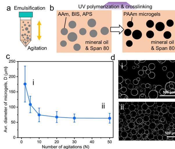
**Fig. 1** Preparation and the size control of PAAm microgels. (a) Water-in-oil emulsification with different droplet sizes controlled by the number of agitations. (b) Polymerization and crosslinking of PAAm precursor droplets by UV irradiation. (c) The effect of the number of agitations ( $N$ ) in average diameters of PAAm microgels ( $D$ ). (d) Thresholded Z-slice optical microscope images of (i) large ( $N = 2$ ) and (ii) small ( $N = 50$ ) microgels, respectively.
