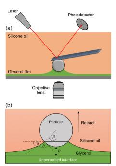
Fig. 1 (a) Colloidal probe experimental setup for a liquid–liquid interface, mounted over a confocal microscope. (b) Schematic image of the experiment showing relevant geometric parameters.  $\theta$  is the contact angle,  $\beta$  is the position of three-phase contact line,  $\alpha$  is the angle between the interface and the horizontal, and D is distance from the unperturbed interface
