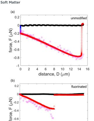
Fig. 5 Comparison of theoretically calculated force and experimentally measured force. (a) Unmodified (hydrophilic) case, (b) fluorinated (hydrophobic) case.
