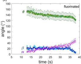
Fig. 4 Distribution of  $\theta$ ,  $\beta$  and  $\alpha$  with respect to time for (a) unmodified (hydrophilic) and (b) fluorinated (hydrophobic) case. Angles are measured for three sets of experiments and error bars represent 10% error.
