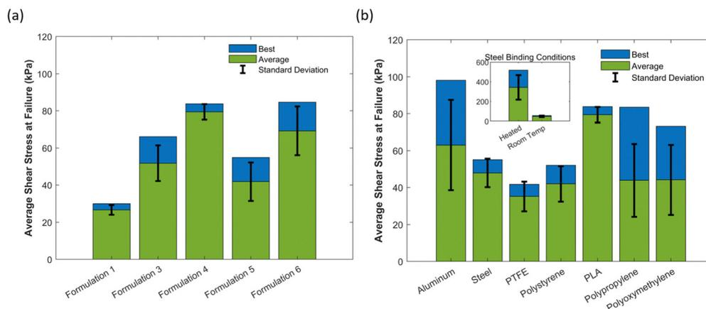
Fig. 3 Average shear stress at failure from lap shear testing (a) for different formulations on PLA laps and (b) of formulation 4 (TMSDA:EDDT (1:0.75) with HEA:BA (80:20)) on different laps.
