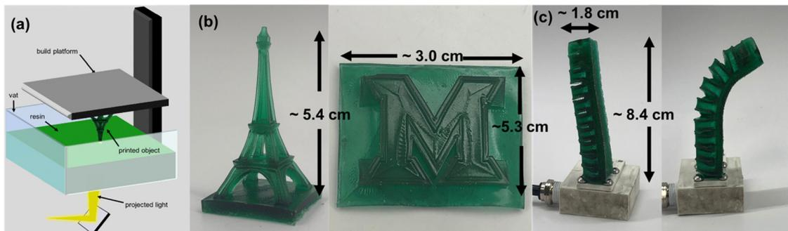
Fig. 4 (a) Schematic of the DLP 3D-printing process used to produce (b) the Eiffel tower, Miami University logo, and (c) a one-piece pneumatic actuator. All prints utilized formulation 4 with HEA : BA (80 : 20) and TMSDA : EDDT (1 : 0.75).
