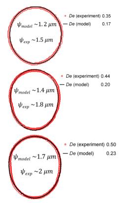
Fig. 7 Experimentally obtained shape of the deformed droplets overlaid with the model prediction for three different values of De.
