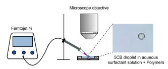
Fig. 2 Schematic representation of the experimental setup along with a micrograph depicting an active droplet with a diameter of 50  $\mu m$ .
