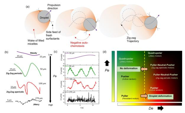
Fig. 11 (a) Schematic depicting the mechanism of zigzag motion of the active 5CB droplet. (b) Droplet trajectory and (c) temporal evolution of their corresponding speed (U) for different droplet sizes in fluid 5. (d) Schematic of proposed phase diagram between Pe\* and De mapping the different modes of droplet swimming under various surroundings.
