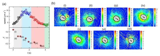
Fig. 10 (a) Variation in speed U and  $\beta$  with time during one persistent stretch of the zigzag motion (b) fluorescent micrographs depicting streamlines obtained from PIV measurements. The streamlines represent the flow-field around the droplet ( $\sim$  50  $\mu$ m) in the laboratory frame for (i) puller (iv) neutral and (vii) pusher swimming modes. Color bars represent the magnitude of the velocity field around the droplet.
