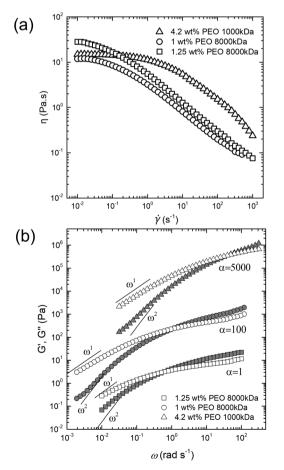
Fig. 4 (a) Flow sweep experiments showing the variation of bulk viscosity  $\eta_0$  with shear rate  $\dot{\gamma}$  and (b) frequency sweep experiments for different polymer solutions carried out at a strain of 1%. Closed symbols and open symbols represent storage  $(G'(\omega))$  and loss moduli  $(G''(\omega))$  respectively.
