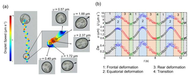
Fig. 9 (a) X-Y trajectory, color-coded by the droplet speed, of an active 5CB droplet (~50 µm) in fluid 5. Enlarged insets are the optical micrographs of droplets at different instances. (b) Corresponding variation in U,  $\psi$  and De with time. Region 1,2 and 3 correspond to frontal, equatorial, rear deformation states respectively. Region 4 corresponds to the transition state with minimum deformation
