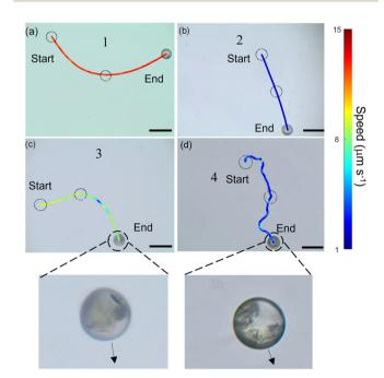
Fig. 3 Representative trajectories, color-coded by the speed of the active 5CB droplets in fluid (a) 1 (b) 2 (c) 3 and (d) 4. The scale bars correspond to 100 µm. The enlarged insets are the optical micrographs demonstrating the deformed shape of the droplet in (c) and the undeformed shape in (d).
