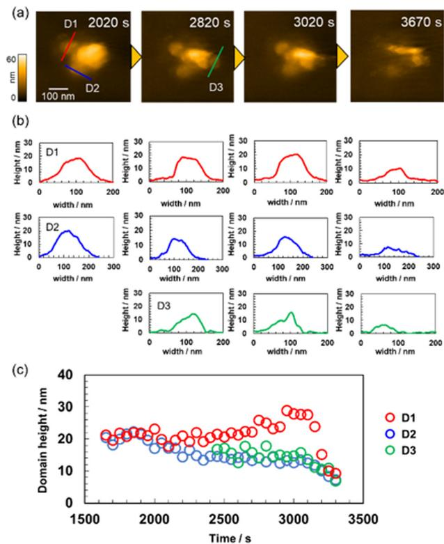
Fig. 6 HS-AFM analysis of the degradation behavior of the spherical degradation products at 30 °C in the presence of 62.5 mM NaIO<sub>4</sub>: (a) height images, (b) cross-sectional profiles corresponding to each line in (a) and (c) changes in the domain size during degradation.
