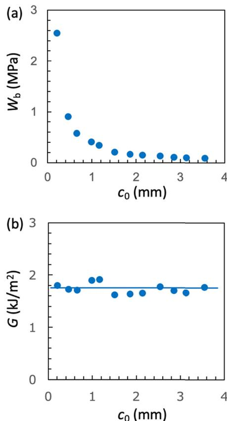
Fig. 2 (a) Strain energy density at break ( $W_b$ ) as a function of the initial notch length ( $c_0$ ) for SBR (non-SIC rubber) at 25 °C and a strain rate of 0.60 s<sup>-1</sup> in the edge-crack test. (b) The  $c_0$  dependence of tearing energy ( $G$ ) calculated using the data in (a) with eqn (2).
