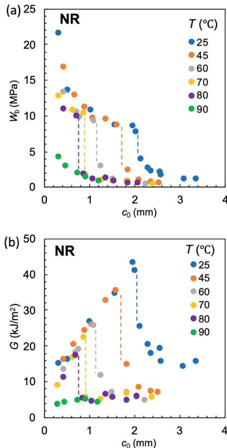
Fig. 4 (a) Strain energy density at break ( $W_b$ ) as a function of the initial notch length ( $c_0$ ) at various ambient temperatures ( $T$ ) for NR-A at a strain rate of 0.5 s<sup>-1</sup>. (b) The  $c_0$  dependence of tearing energy ( $G$ ) calculated using the data in (a) with eqn (2). The dashed lines indicate the position of  $c_0^*$  at which an abrupt change occurs for each  $T$ . No abrupt change is observed at 90 °C.
