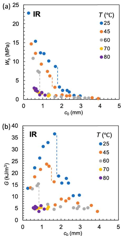
Fig. 5 (a) Strain energy density at break ( $W_b$ ) as a function of the initial notch length ( $c_0$ ) at various ambient temperatures ( $T$ ) for IR-A at a strain rate of  $0.5 \text{ s}^{-1}$ . (b) The  $c_0$  dependence of tearing energy ( $G$ ) calculated using the data in (a) with eqn (2). The dashed lines indicate the position of  $c_0^*$  at which an abrupt change occurs for each  $T$ . No abrupt change is observed at  $T \geq 70 \text{ }^\circ\text{C}$ .
