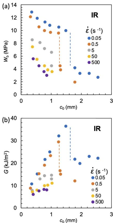
Fig. 9 (a) Strain energy density at break ( $W_b$ ) as a function of the initial notch length ( $c_0$ ) at various strain rates ( $\dot{\epsilon}$ ) for IR-A at 25 °C. (b) The  $c_0$  dependence of tearing energy ( $G$ ) calculated using the data in (a) with eqn (2). The dashed lines indicate the position of  $c_0^*$  at which an abrupt change occurs for each  $\dot{\epsilon}$ . No abrupt change is observed at  $\dot{\epsilon} > 5 \text{ s}^{-1}$ .
