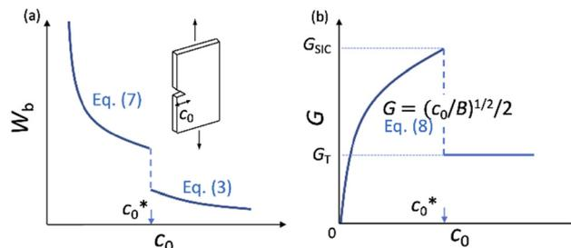
Fig. 1 Schematic illustrations of the theoretical relationships of (a) strain energy density at break ( $W_b$ ) and initial notch length ( $c_0$ ), and (b) tearing energy ( $G$ ) and  $c_0$ . Crack growth of a single-edge crack specimen (inset) undergoes a transition between the catastrophic failure ( $c_0 > c_0^*$ ) and the  $dc/dn$  mode ( $c_0 < c_0^*$ ).
