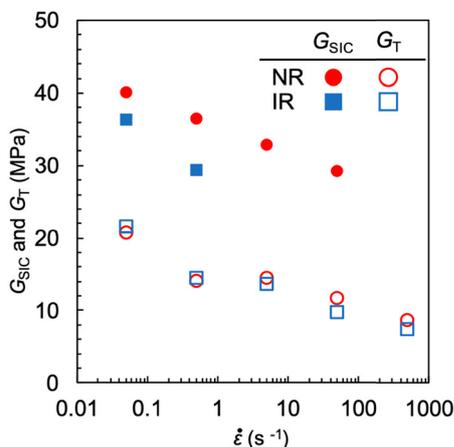
Fig. 10 Strain rate dependence of the tearing energy *via* the SIC-reinforcement effect ( $G_{\text{SIC}}$ ) and the tearing energy in catastrophic failure ( $G_{\text{T}}$ ) for NR-A and IR-A. The SIC-reinforcement effect vanishes at  $\dot{\epsilon} > 50 \text{ s}^{-1}$  and  $\dot{\epsilon} > 0.5 \text{ s}^{-1}$  for NR-A and IR-A, respectively.
