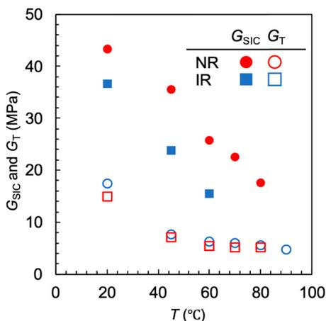
Fig. 6 Temperature dependence of the tearing energy *via* the SIC-reinforcement effect ( $G_{\text{SIC}}$ ) and the tearing energy in catastrophic failure ( $G_{\text{T}}$ ) for NR-A and IR-A. The SIC-reinforcement effect vanishes at  $T > 80 \text{ }^\circ\text{C}$  and  $T > 60 \text{ }^\circ\text{C}$  for NR-A and IR-A, respectively.
