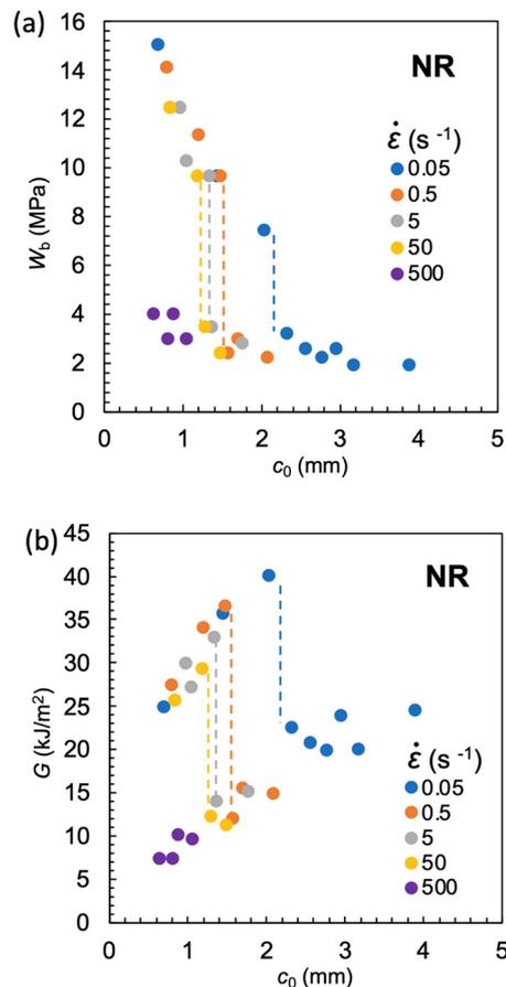
Fig. 8 (a) Strain energy density at break ( $W_b$ ) as a function of the initial notch length ( $c_0$ ) at various strain rates ( $\dot{\epsilon}$ ) for NR-A at 25 °C. (b) The  $c_0$  dependence of tearing energy ( $G$ ) calculated using the data in (a) with eqn (2). The dashed lines indicate the position of  $c_0^*$  at which an abrupt change occurs for each  $\dot{\epsilon}$ . No abrupt change is observed at 500 s<sup>-1</sup>.
