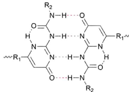
Fig. 4 Chemical structure of a dimerised 2-ureido-4[1H]-pyrimidinone (UPy) motif through quadruple hydrogen bonding.
