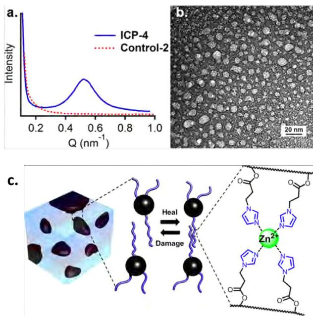
Fig. 9 (a) SAXS and (b) TEM results, showing phase separation for (c)  $\text{Zn}^{2+}$ -imidazole crosslinked polymers. Reprinted with permission from ref. 112 Copyright 2014 American Chemical Society.
