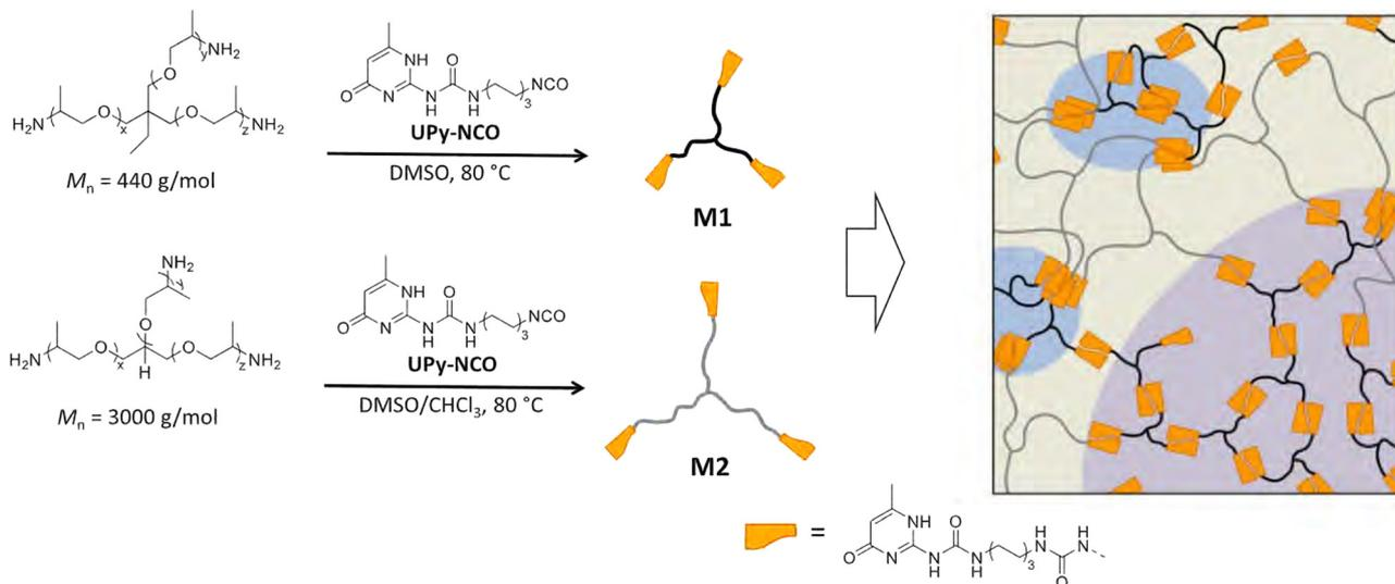
**Fig. 6** A schematic showing the three distinct phases formed through combining smaller (M1) and larger (M2) trifunctionalised poly(propylene oxide) monomers. The distinct phases are rich in (1) mainly M2 monomers (tan), (2) mainly M1 monomers (purple) or (3) crystalline UPy dimers (blue). Reprinted with permission from ref. 97 Copyright 2019 American Chemical Society.
