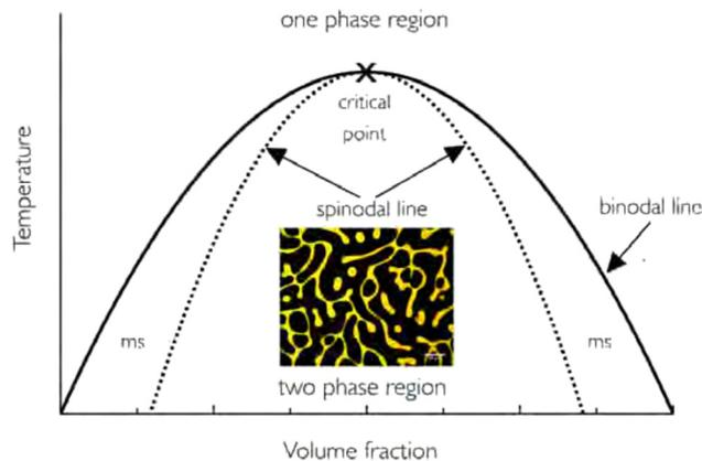
**Fig. 1** Example of a phase diagram for a polymer–solvent system. The binodal line separates the one-phase region with the phase-separated two-phase region. The metastable (ms) region lies between the binodal and spinodal regions. The included image corresponds to spinodal decomposition of the system. Note that in reality, for most polymer solutions, the phase diagram is often asymmetric. Reprinted with permission from ref. 12 Copyright 2018 IOP Publishing Ltd.
