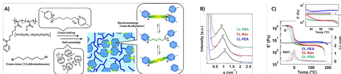
Fig. 18 (A) Overview of the formation of *trans*-*N*-alkylation-based polyacrylate CANs with either ethyl (CL-PEA), butyl (CL-PBA) or blended ethyl and butyl (CL-Ran) alkyl chains. (B) SAXS results of the CANs. (C) Temperature sweep results, showing  $\tan(\delta)$  and  $E'$  curves. Reprinted (adapted) with permission from ref. 192 Copyright 2022 American Chemical Society.
