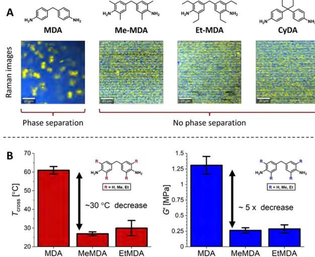
Fig. 14 (A) Raman images of polyimine CANs synthesised from MDA monomers with different sterically demanding groups, (B)  $T_{\text{cross}}$  (where  $\tan(\delta) = 1$ ) and  $G'$  of the materials with either MDA ( $R = H$ ), MeMDA ( $R = Me$ ) or EtMDA ( $R = Et$ ) as dianiline monomers. Reprinted (adapted) with permission from ref. 66 Copyright 2022 American Chemical Society.
