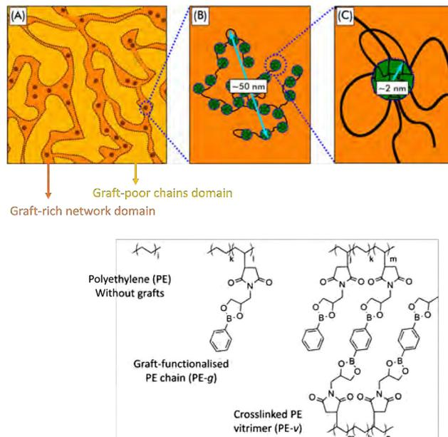
Fig. 19 Schematic overview of phase-separated boronic ester grafted PE CANs into graft-rich and graft-poor domains. Reprinted (adapted) with permission from ref. 193. Copyright 2020 American Chemical Society.
