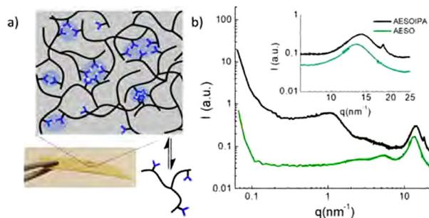
Fig. 3 SAXS–WAXS spectra of acrylated epoxidised soybean oil and isophthalic acid (IPA) functionalised soybean oil. IPA-rich domains cause a diffraction peak around  $1.5 \text{ nm}^{-1}$  due to microphase separation, and a sharp band at  $18.5 \text{ nm}^{-1}$  suggesting  $\pi$ – $\pi$  stacking of IPA motifs. Reprinted with permission from ref. 71 Copyright 2019 American Chemical Society.
