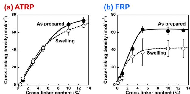
Fig. 1 The effect of the cross-linker content on the cross-linking density of the PNIPAAm gels (●, as-prepared; ○, swollen) synthesized *via* ATRP (a) and FRP (b). The cross-linking densities were determined from the compression modulus.
