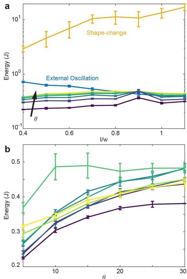
Fig. 8 Comparing energy usage between procedures. (a) Comparisons of energy output for different procedures as a function aspect ratio. The internally-oscillated data are the unlabeled lines where  $\theta$  is varied. All data points are averaged from three trials. (b) Energy usage for the internal oscillation procedure as a function of  $\theta$  for various aspect ratios. The color gradient here mirrors that used in the earlier figures with purple to yellow being high to low  $l/w$ .
