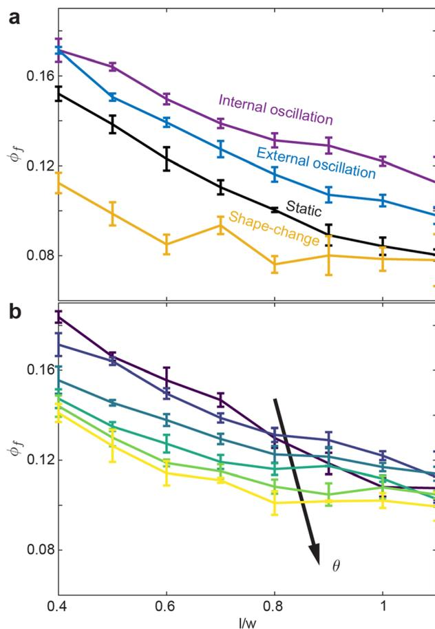
**Fig. 7** Final volume fraction  $\phi_f$  for the various procedures. (a)  $\phi_f$  versus  $l/w$  for all procedures. For the internally-oscillated procedure,  $\theta = 10^\circ$  was used. (b)  $\phi_f$  versus aspect ratio for the internally-oscillated system, each line is has a different  $\theta \in [5^\circ, 30^\circ]$   $\theta \in [5^\circ, 30^\circ]$ .
