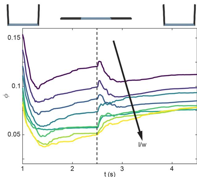
Fig. 5 Evolution of  $\phi$  at different  $l/w \in [0.4, 1.1]$  for the shape-change procedure. Time evolution of  $\phi$  for varying  $l/w$  performing the shape-change procedure. The vertical dashed line represents when the “straight” to “u” configuration change begins.
