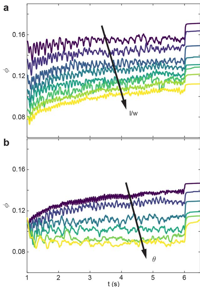
**Fig. 6** Time evolution of volume fraction  $\phi$  for various  $l/w$  and  $\theta$  for the internally-oscillated procedure. (a)  $l/w$  is varied  $\in [0.4, 1.1]$  while  $\theta = 10^\circ$  is held constant. (b)  $\theta$  is varied  $\in [5^\circ, 30^\circ]$  while  $l/w = 0.7$  is held constant.
