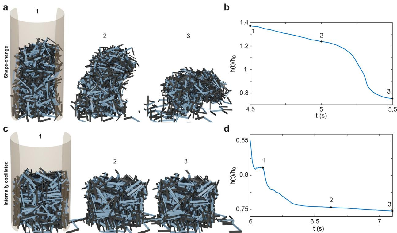
**Fig. 10** “Tumbling” and “melting” behavior for active procedures. (a and c) Renders of a shape-change trial and internally-oscillated trial, respectively, at three instances instances. (b and d) The z-plane center-of-mass (CoM) of the collective vs. time, where the three renders from (a and c) are indicated with black points.
