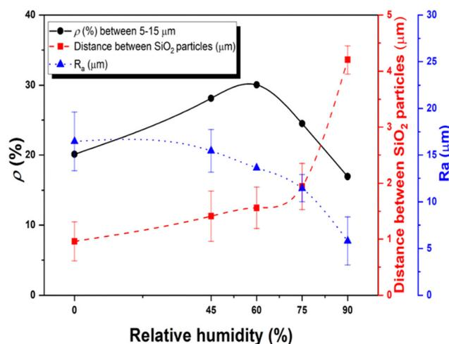
Fig. 3 Relationship between the percentage of infrared radiation emitted by the human body that is reflected by the PNIPAM-based hydrogel composite containing 20 wt% of SiO<sub>2</sub> (black circles), the distance between the SiO<sub>2</sub> particles (red squares) and the surface roughness (blue triangles) with respect to the relative humidity.
