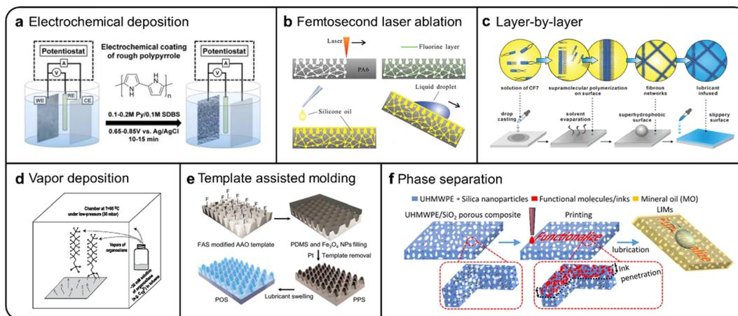
Fig. 5 Schematic diagram of different preparation methods of the SLIPS. (a) Electrochemical deposition process.<sup>48</sup> (b) Femtosecond laser ablation.<sup>52</sup> (c) Layer-by-layer deposition.<sup>50</sup> (d) Vapor deposition process.<sup>53</sup> (e) Template assisted molding.<sup>54</sup> (f) Phase separation.<sup>55</sup>
