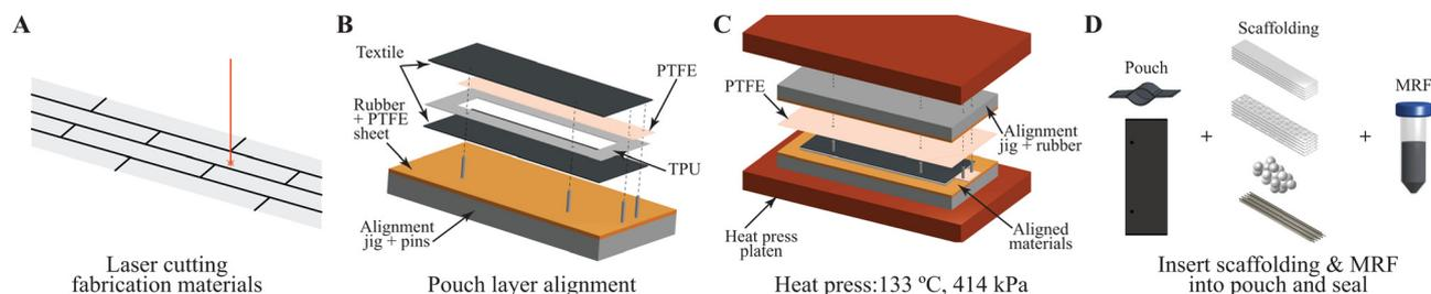
Fig. 3 Fabrication of MRJ beams process. (A) Materials are laser cut to size. (B) Textile, TPU, and PTFE are aligned to create the pouch of the beam. (C) Pouch elements are bonded on the heat press for 4 min. (D) Scaffolding material and 1 mL of magnetorheological fluid (MRF) are inserted into the pouch, which is then hand-sealed.
