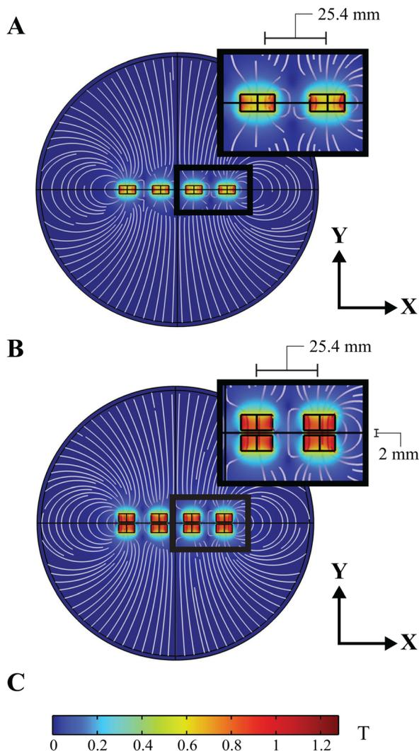
Fig. 4 COMSOL simulations of (A) one row and (B) two rows of neodymium magnets in the 2 mm spacing case with the magnetic field lines in white and  $xy$  reference frames. (C) shows the magnetic flux density norm that applies to (A) and (B).
