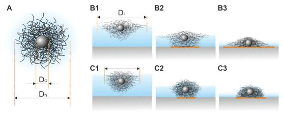
Fig. 8 (A) Schematic illustration of the structure of a CS microgel.  $D_c$  denotes the diameter of the core and  $D_h$  the hydrodynamic diameter. (B1-B3) CS microgels with high deformability adsorbed at the air/water interface at three different drying stages. D<sub>i</sub> denotes the diameter at the interface and the orange area depicts the contact area between the microgel and the substrate. (C1-C3) the same set of illustrations for CS microgels with low deformability.
