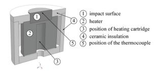
(b) Sectional view of the heating system.
