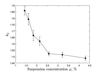
Fig. 11 Dependence of the dimensionless empirical constant  $k_{w_{ij}}$  defined in eqn (25), on the solid phase volume concentration  $\varphi$  in the suspension. The error bars represent one standard deviation.
