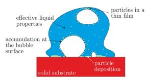
Fig. 2 Assumed phenomena associated with the particulate phase in a suspension drop on a hot substrate, which potentially influence the thermodynamic and hydrodynamic phenomena in the drop.
