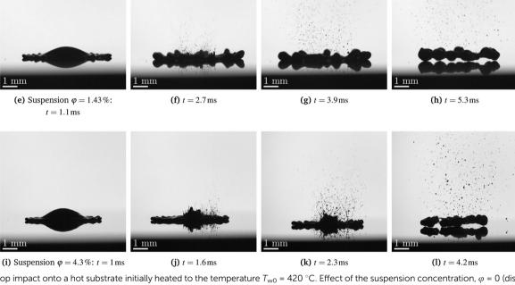
Fig. 12 Drop impact onto a hot substrate initially heated to the temperature  $T_{w0}$  = 420 °C. Effect of the suspension concentration,  $\varphi$  = 0 (distilled water) (a-d),  $\varphi = 1.43\%$  (e-h) and  $\varphi = 4.3\%$  (i-l) on the regime of drop impact. The initial drop diameter  $d_0 = 2.3$  mm and impact velocity  $U_0 = 1.7$  m s<sup>-1</sup> are the same for all the cases. The corresponding videos are available on Zenodo. 46
