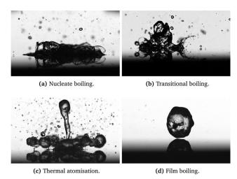
Fig. 1 Typical regimes observed for an impact of a distilled water drop onto a hot substrate. The impact parameters are  $d_0 = 2.3$  mm, impact velocity  $U_0 = 1 \text{ m s}^{-1}$  at various initial wall temperatures, respectively (a) 170 °C, (b) 240 °C, (c) 340 °C, and (d) 420 °C.
