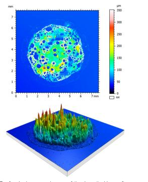
Fig. 9 Confocal microscope images of the deposited layer after suspension drop ( $\varphi$  = 4.3%) impact onto a hot substrate. The parameters of impact correspond to the case shown in Fig. 4(i)-(l).
