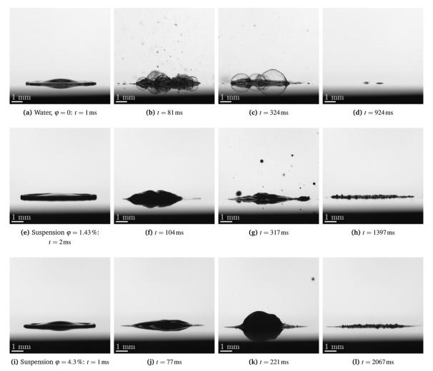
Fig. 4 Drop impact in the nucleate boiling regime. Effect of the suspension concentration,  $\varphi = 0$  (distilled water) (a–d),  $\varphi = 1.43\%$  (e–h) and  $\varphi = 4.3\%$ (i–l) on the drop splash and evaporation. The initial substrate temperature  $T_{w0} = 150$  °C, drop diameter  $d_0 = 2.3$  mm and impact velocity  $U_0 = 1.7$  m s<sup>-1</sup> are the same for all the cases. The corresponding videos are available on Zenodo. 46
