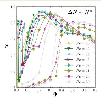
Fig. 9 Plot of the exponent  $\alpha$  of the relation  $\Delta N \sim \bar{N}^{\alpha}$  as a function of the packing fraction  $\Phi$  for Pe = 10, 12, 14, 16, 18, 21, 25 and 30 with  $\zeta_{\rm tr}$  = 15.4 and  $\zeta_{rot} = -0.38$  (continuous lines) and for ABPs with periodic boundary conditions at Pe = 21, 25 and 30 (dashed lines).
