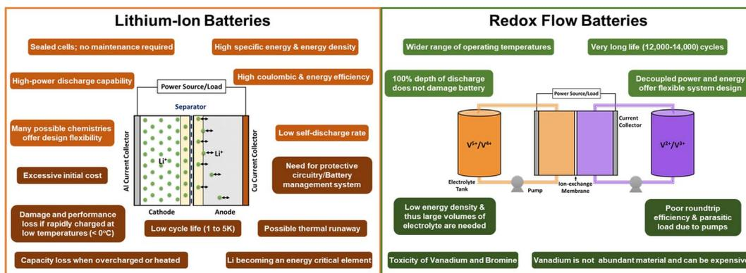
Fig. 4 Comparison of lithium-ion and redox flow batteries.
