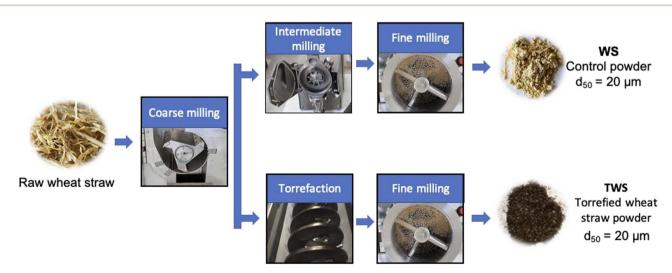
Fig. 1 Technological process routes for the production of control (WS) and torrefied wheat straw (TWS).
