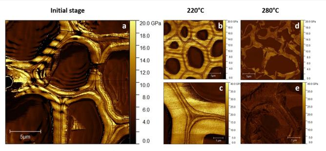
Fig. 3 Indentation modulus mapping for control (WS) wheat straw cell walls (a), treated at 220 °C (b) and 280 °C (d). A focus on the middle lamellae region is also proposed on 220 °C (c) and 280 °C (e) samples.
