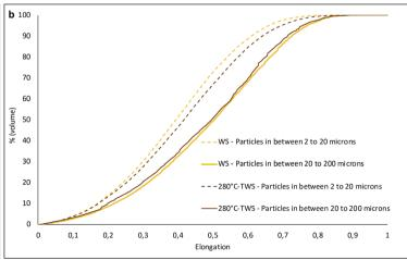
Fig. 5 Particle size distribution (a) and cumulative elongation distribution for particles below 20 μm (b) for control (WS) and torrefied wheat straw (TWS) after milling
