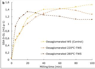
Fig. 4 Evolution of specific surface area before (plain line, Fig. 2a)) and after (dashed line, Fig. 2b) de-agglomeration with ultrasonic treatment (UT) in control (WS) and torrefied samples (220 °C TWS and 280 °C-TWS) in a lab-scale MM400 ball-mill.
