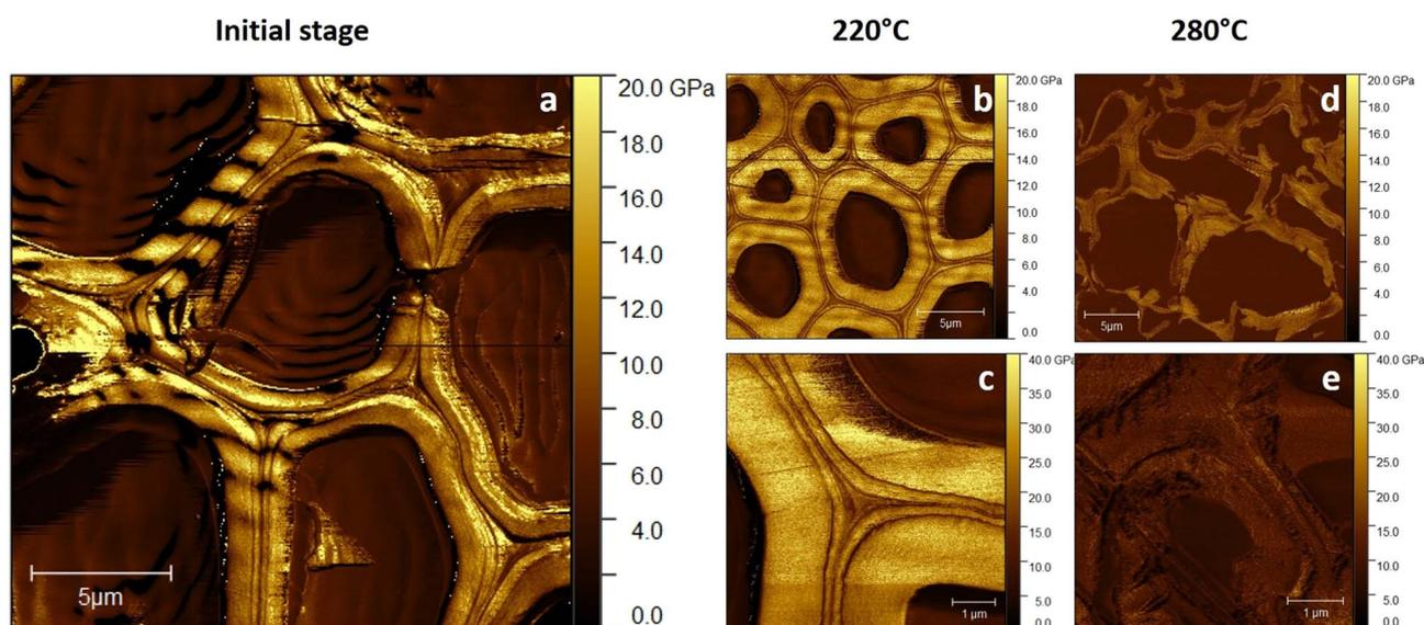
**Fig. 3** Indentation modulus mapping for control (WS) wheat straw cell walls (a), treated at 220 °C (b) and 280 °C (d). A focus on the middle lamellae region is also proposed on 220 °C (c) and 280 °C (e) samples.
