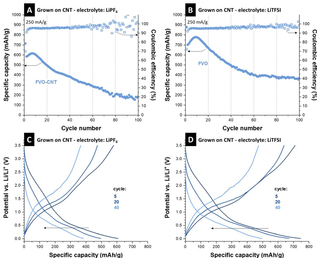
Fig. 4 Stability performances of FVO electrodes at the specific current of 250 mA g<sup>-1</sup> in (A) 1 M LiPF<sub>6</sub> in EC/DMC, and (B) 2 M LiTFSI in EC/DMC with their Coulombic efficiencies, and (C) and (D) their respective charge–discharge curves at cycles 5, 20, and 40.
