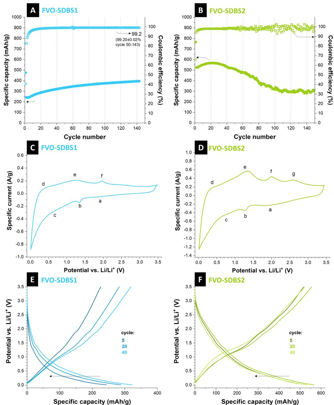
Fig. 5 (A) and (B) Stability of FVO-SDBS1 and FVO-SDBS2 at the specific current of  $250 \text{ mA g}^{-1}$ , respectively. (C) and (D) The respective cyclic voltammetry at the scanning rate of  $0.1 \text{ mV s}^{-1}$ , and (E) and (F) the respective galvanostatic charge-discharge curves.
