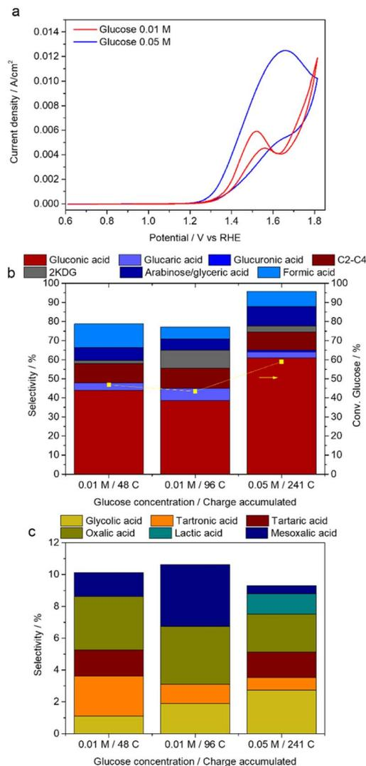
Fig. 6 Comparison of the electrooxidation of 0.01 and 0.05 M glucose in NaOH 0.1 M. (a) CV recorded in the 0.61–1.81 V vs. RHE range with a scan rate of 5 mV s<sup>-1</sup>; (b and c) results obtained during the electrolysis at 1.81 V vs. RHE, (b) glucose conversion and selectivity in the main reaction products and by-products; (c) selectivity in C2–C4.
