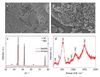
Fig. 1 Characterization of the NiO/Ni sample: (a) SEM image at low magnification; (b) SEM image at high magnification; (c) XRD pattern, for comparison the pattern of a non-calcined Ni foam (Ni-bare); (d) micro-Raman spectra.
