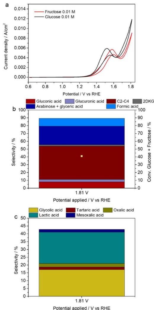
**Fig. 7** Electroactivity of a fructose 0.01 M in NaOH 0.1 M electrolyte. (a) CV recorded in the 0.61–1.81 V vs. RHE range with a scan rate of  $5 \text{ mV s}^{-1}$ , for comparison purposes the CV in a glucose 0.01 M in NaOH 0.1 M electrolyte was included; (b and c) results obtained during the electrolysis at 1.81 V vs. RHE, glucose + fructose conversion and selectivity in the reaction products. Charge accumulated 48 C.
