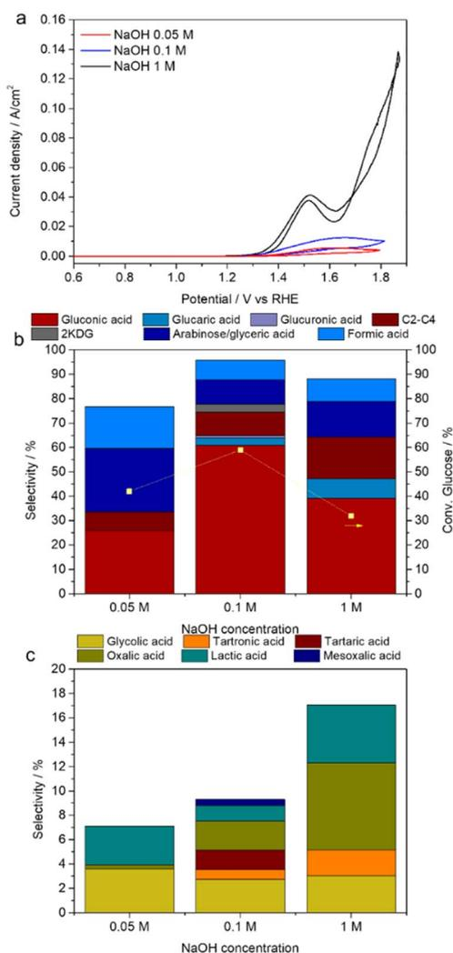
Fig. 10 Effect of the NaOH concentration on the electrooxidation of a 0.05 M glucose solution. (a) CVs recorded in the 0.61–1.81 V vs. RHE range with a scan rate of 5 mV s<sup>−1</sup>; (b and c) conversion and selectivity in the reaction products obtained at an applied potential of 1.81 V vs. RHE and 241 C accumulated.
