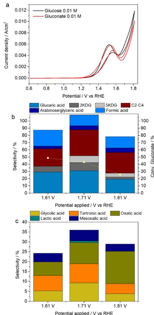
**Fig. 8** Electroactivity of a gluconate 0.01 M in NaOH 0.1 M electrolyte. (a) CVs recorded in the 0.61–1.81 V vs. RHE range with a scan rate of  $5 \text{ mV s}^{-1}$ , for comparison purposes the CV in a glucose 0.01 M in NaOH 0.1 M electrolyte was included; (b and c) results obtained during the electrolysis at 1.61, 1.71, and 1.81 V vs. RHE, gluconate conversion and selectivity in the reaction products. Charge accumulated 96 C.
