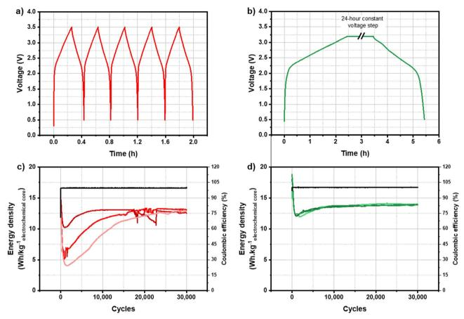
Fig. 1 Voltage profiles at room temperature during CC formation (a) and CV formation (b) and energy densities and coulombic efficiency during long-term cycling at 16 mA cm $^{-2}$  between 0.5 and 3.5 V in the pouch cell configuration after CC formation (c) and CV formation (d).
