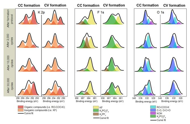
Fig. 6 High-resolution K 2p, F 1s and O 1s XPS spectra obtained on the graphite electrode surface after CC formation and CV formation, after 2000, 10 000 and 30 000 cycles at 16 mA cm $^{-2}$  at room temperature.
