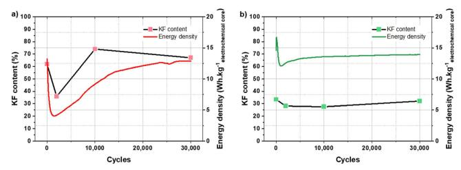
Fig. 8 Evolution of KF content in the SEI and energy density of a KIC cell during cycling at 16 mA cm<sup>-2</sup> at room temperature after CC formation (a) and after CV formation (b).
