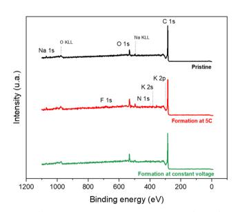
Fig. 3 XPS survey spectra of a pristine graphite electrode (in black) and a graphite electrode after CC formation (in red) and after CV formation (in green).
