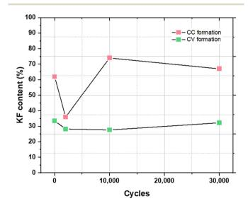
Fig. 7 Evolution of KF content in the SEI for each cycling step after CC formation (in red) and after CV formation (in green).
