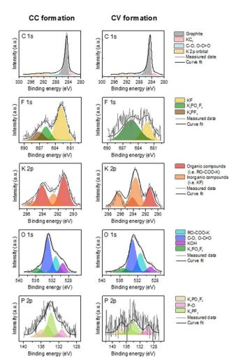
Fig. 4 High-resolution C 1s K 2p, F 1s, K 2p, O 1s and P 2p XPS spectra obtained on the graphite electrode surface after CC formation and CV
