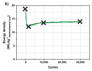
Fig. 5 Long-term cycling of a hybrid KIC in  $0.8 \text{ mol L}^{-1} \text{ KPF}_6 \text{ AN}$  at  $16 \text{ mA cm}^{-2}$  between 0.5 and 3.5 V at room temperature in the pouch cell configuration after CC formation (a) and after CV formation (b).8
