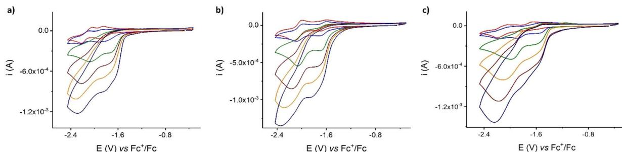
Fig. 5 Cyclic voltammograms of 1 mM of catalysts C2 (a), C3 (b) and C4 (c) recorded in  $\text{CH}_3\text{CN}$  with  $0.1 \text{ M TBAPF}_6$  at  $30 \text{ V s}^{-1}$  with glassy carbon as working electrode and increasing amounts of TFA (0 red, 1 blue, 5 green, 10 brown, 15 orange and 20 navy blue mM).
