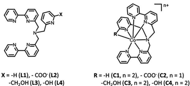
Fig. 1 Structures of the ligands **L1**–**L4** (left) and the corresponding Co complexes (**C1**–**C4**). For the sake of clarity, the description of the different counterions of the complexes is provided in the text.
