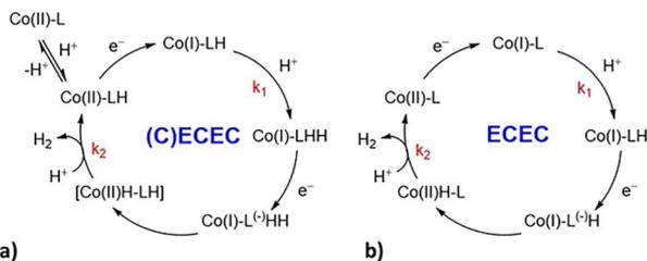
**Scheme 1** Proposed pathways for H<sub>2</sub> evolution under electrochemical conditions in acetonitrile solution with TFA as the proton source: (a) (C)ECEC for complexes C2 and C4; (b) ECEC mechanism for complexes C3 and C1.<sup>27</sup>
