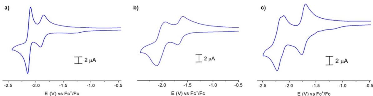
Fig. 4 Cyclic voltammograms (CVs) of 1 mM solutions of complexes (a: C2, b: C3, c: C4) recorded at  $0.1 \text{ V s}^{-1}$  in  $\text{CH}_3\text{CN}$  with  $0.1 \text{ M TBAPF}_6$ , with glassy carbon as working electrode.
