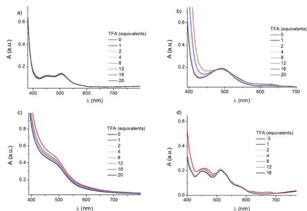
Fig. 3 UV-Vis spectra of 4 mM solutions of complexes **C1** (a), **C2** (b), **C3** (c), and **C4** (d) in CH<sub>3</sub>CN at increasing amounts of TFA keeping the final volume (2 mL) unchanged.
