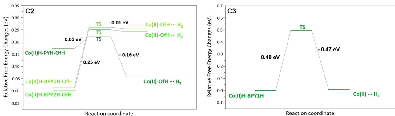
Fig. 10 Calculated free energy profiles ( $\Delta G$ ) starting from the second protonation step until formation of  $\text{H}_2$ , for C2 (left) and C3 (right). At this step, once formed,  $\text{H}_2$  is still in interaction with the complex (see structures in Fig. ES26†). The structures corresponding to stationary points (minima and transition states, TS) are given in Fig. ES26,† including the imaginary frequency of the most relevant TSs.
