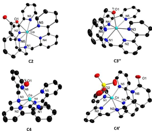
Fig. 2 Crystal structures of complexes **C2**, **C3''** and the two tautomers **C4** (enol form) and **C4'** (keto form). Colour code: Co (turquoise), N (blue), O (red), C (black), S (yellow), H (white). Non-coordinating counterions (*i.e.*, BF<sub>4</sub><sup>-</sup>, PF<sub>6</sub><sup>-</sup> and SO<sub>4</sub><sup>2-</sup>), solvents, and other hydrogen atoms have been omitted for clarity.
