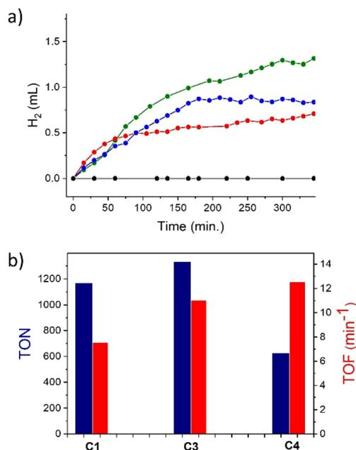
Fig. 7 (a)  $\text{H}_2$  evolution in mL over time for solutions of 5  $\mu\text{M}$  catalysts C1 (blue), C3 (green), and C4 (red) and without catalysts (black). The experiments were performed in 1.0 M acetate buffer at pH 4.0 with 0.1 M ascorbic acid and 0.5 mM  $[\text{Ru}(\text{bpy})_3]\text{Cl}_2$  at 20 °C and the solutions were irradiated with LED light at 475 nm. (b) Maximum TONs and TOFs for C1, C3 and C4.
