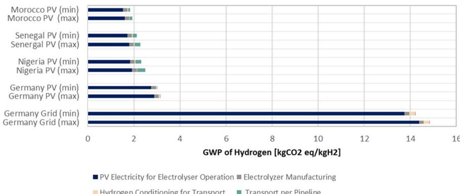
Fig. 8 Scenario analysis for different insulation levels and electrolyzer consumption. GWP of PV-powered hydrogen production by country with high-efficiency scenario (power consumption: 55 kW h per kg H<sub>2</sub>) and low-efficiency (electricity demand of 57.5 kW h per kg H<sub>2</sub>). Blue – GWP caused by PV electricity, grey – GWP of plant manufacturing, beige – GWP of compression and conditioning, and mint – the pipeline transport.
