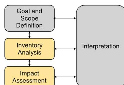
Fig. 2 Schematic illustration of the life cycle assessment framework.
