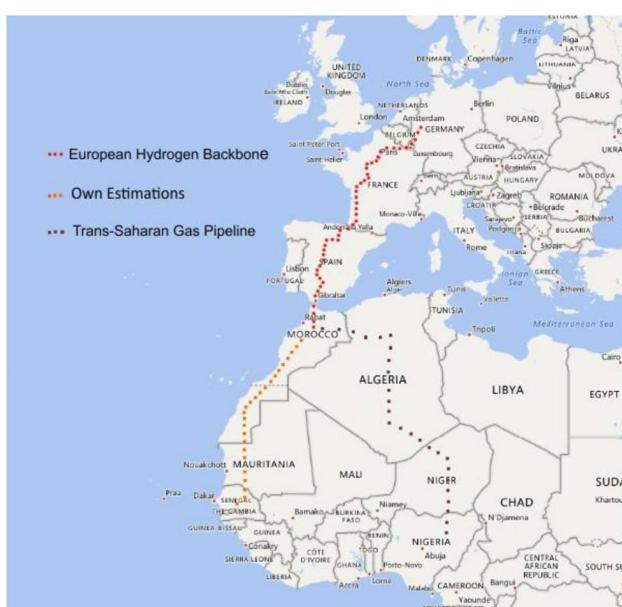
Fig. 1 Hydrogen supply chain. Red-colored route is possible corridor for German imports based on existing natural gas infrastructure (European Hydrogen Backbone).<sup>28</sup> The routes in Africa are estimated on the basis of our own calculations and the planned Trans-Saharan Gas Pipeline project.
