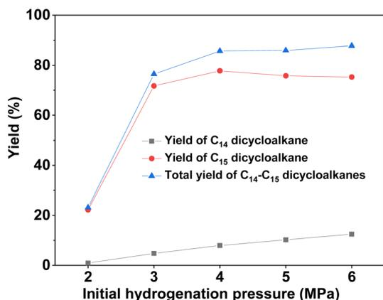
Fig. 10 Yields of different dicycloalkanes from the HDO of **1A** over the Ru/H-ZSM-5 catalyst as a function of the initial hydrogen pressure at room temperature. Reaction conditions: 5 h, 473 K; 0.2 g **1A**, 0.1 g catalyst; 40 mL cyclohexane was used for each test.
