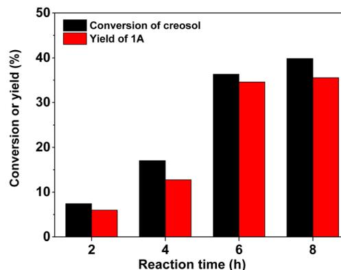
Fig. 3 Creosol conversions and the yields of **1A** over the 40% HPW/ $\text{SiO}_2$  catalyst as a function of the reaction time. Reaction conditions: 323 K; 20 mmol creosol, 10 mmol formaldehyde, and 0.05 g catalyst were used in each test.
