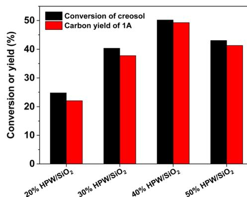
Fig. 2 Creosol conversions and the yields of **1A** over the HPW/ $\text{SiO}_2$  catalysts. Reaction conditions: 333 K, 2 h; 25 mmol creosol, 10 mmol formaldehyde and 0.1 g catalyst were used in each test.
