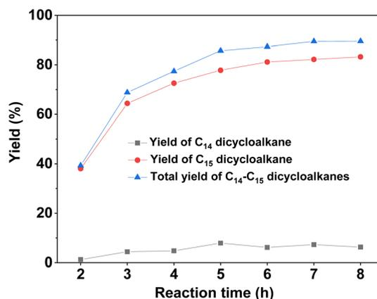
Fig. 11 Yields of different dicycloalkanes from the HDO of **1A** over the Ru/H-ZSM-5 catalyst as a function of the initial hydrogen pressure at room temperature. Reaction conditions: 4 MPa  $\text{H}_2$ , 473 K; 0.2 g **1A**, 0.1 g catalyst; 40 mL cyclohexane was used for each test.
