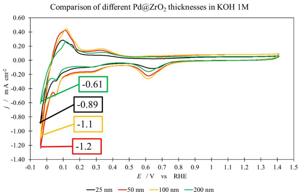
Fig. 5 Cyclic voltammetry in aqueous 1 M KOH for different thicknesses of the deposit. Scan rate: 20 mV s<sup>-1</sup>, electrode geometric area: 1 cm<sup>2</sup>.
