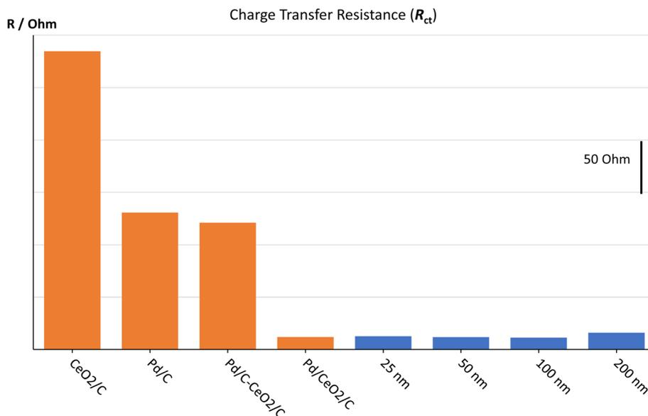
**Fig. 9** Charge transfer resistances of 4 different ceria-based composite materials (from Vizza *et al.*<sup>5</sup> – orange bars) and 4 different thicknesses of Pd@ZrO<sub>2</sub> (blue bars), in KOH 1 M at −275 mV vs. RHE. Pd/C–CeO<sub>2</sub>/C denote a mix of 2 co-deposited powders: Pd/C and CeO<sub>2</sub>/C. Pd/CeO<sub>2</sub>/C denote a co-synthesis of Pd and ceria oxide.
