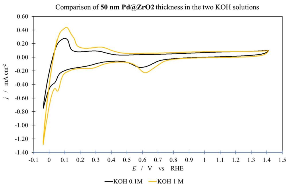
Fig. 6 Cyclic voltammetry in aqueous KOH solutions of Pd@ZrO<sub>2</sub> 50 nm layer deposited by IBS on FTO. Scan rate: 20 mV s<sup>-1</sup>, electrode geometric area: 1 cm<sup>2</sup>.
