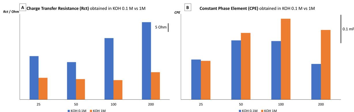
Fig. 8 (A) Charge transfer resistances ( $R_{ct}$ ). (B) Constant phase element (CPE) for 25, 50, 100, and 200 nm thickness of Pd@ZrO<sub>2</sub> layers sputtered onto FTO, in 0.1 M KOH (blue bar) and 1 M KOH (orange bar). These values are obtained from the fitting of EIS data presented in Fig. 7. The maximum iterations are 1000, type of fitting is complex, GDAE. Accuracy is 2.
