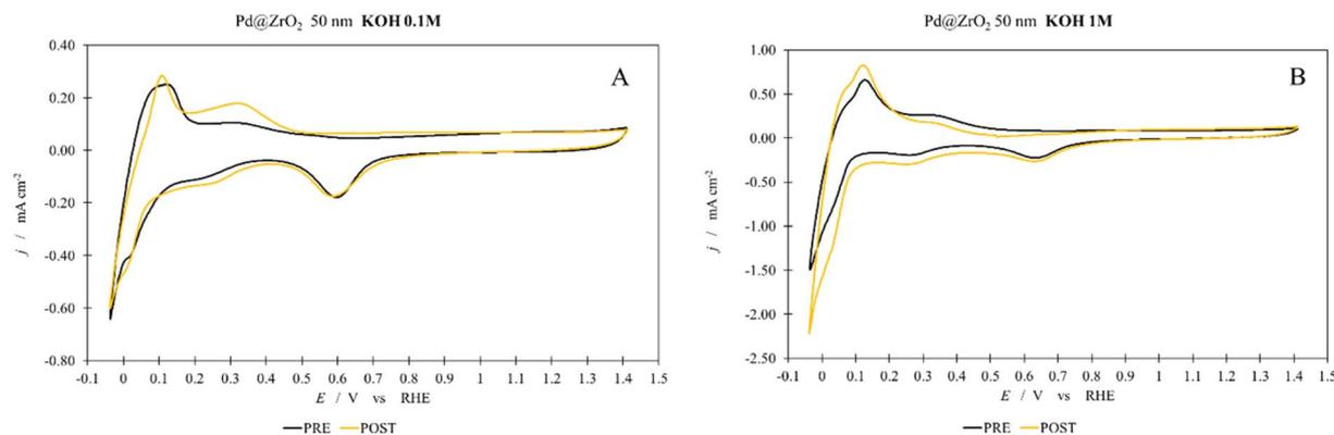
Fig. 10 CV of a 50 nm Pd@ZrO<sub>2</sub> electrode in 0.1 M KOH, (A), and 1 M KOH, (B), pre and post 5000 CV cycles. Scan rate: 20 mV s<sup>-1</sup>, electrode geometric area: 1 cm<sup>2</sup>.
