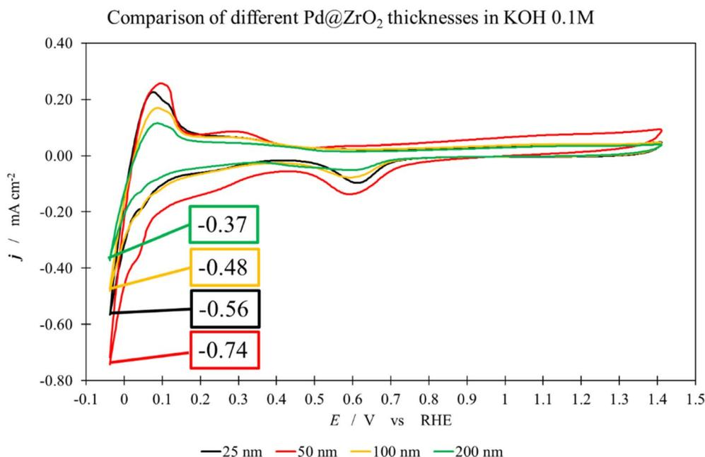
Fig. 4 Cyclic voltammetry in aqueous 0.1 M KOH for different thicknesses of the deposit. Scan rate: 20 mV s<sup>-1</sup>, electrode geometric area: 1 cm<sup>2</sup>.
