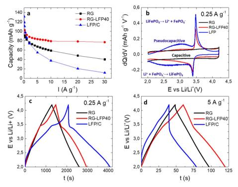
Fig. 6 Dependence of the specific capacitance on the current density (a), differential capacity vs. voltage plot (b), galvanostatic charge/discharge profiles registered at 0.25 A  $g^{-1}$  (c), and 5 A  $g^{-1}$  (d) for the studied samples.
