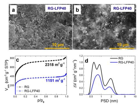
Fig. 5 EDT and BSD SEM images of RG-LFP40 electrodes (a and b), N<sub>2</sub> adsorption/desorption isotherms (c), and pore size distribution of RG and RG-LFP40 (d).
