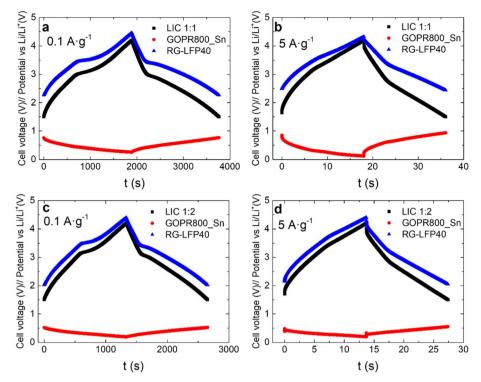
Fig. 7 Galvanostatic charge/discharge profiles at 0.1 A g<sup>-1</sup> and 5 A g<sup>-1</sup> for LIC1:1 (a and b) and LIC1:2 (c and d): LIC (black), negative electrode (red), and positive electrode (blue).
