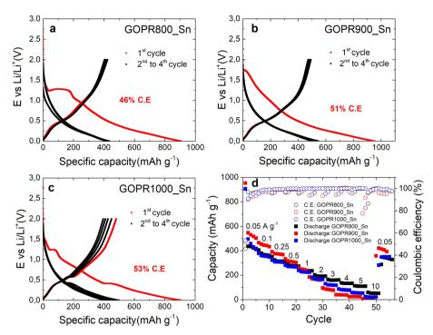
Fig. 3 Electrochemical characterization of the negative electrodes: galvanostatic charge/discharge of the first four cycles recorded at  $0.05 \,\mathrm{A\,g^{-1}}$ for GOPR800\_Sn (a), GOPR900\_Sn (b), GOPR1000\_Sn (c) and rate capability and their respective coulombic efficiency (d).
