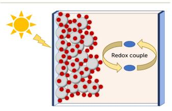
Fig. 2 Schematics of a liquid DSSC. The mesoporous semiconductor (grey discs) is sintered on a conductive substrate and the dye (red discs) is adsorbed on its surface. A solution of the redox couple fills the space between the electrodes.
