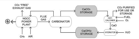
Fig. 1 Schematic of the highly flexible backup NGCC power plant with CO<sub>2</sub> capture using a CaO/Ca(OH)<sub>2</sub>/CaCO<sub>3</sub> loop, including Ca(OH)<sub>2</sub> and CaCO<sub>3</sub> storage silos
