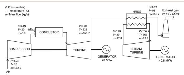
Fig. 2 Simplified schematic of the reference NGCC. Reported pressure (P in bar), temperature (T in °C), and mass flow (m in kg s<sup>-1</sup>).
