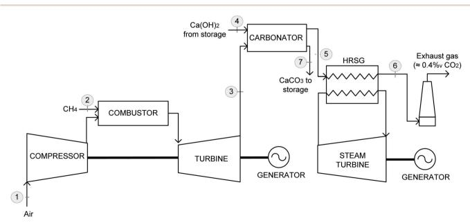
Integration proposed for the CO<sub>2</sub> capture system in the backup NGCC power plant.
