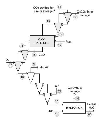
Fig. 5 Sorbent regeneration proposed for the backup CO<sub>2</sub> capture system including the oxy-calcination of the carbonated sorbent (in grey) and the hydration of the CaO (in white).
