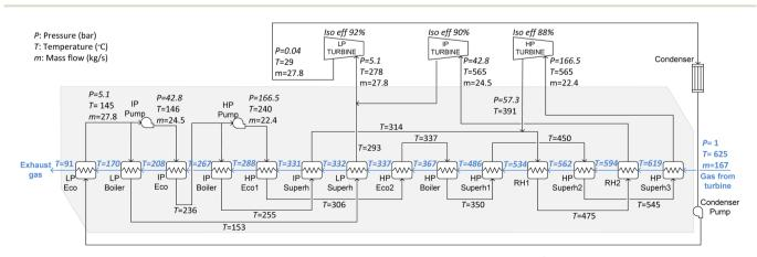
Fig. 3 Reference HRSG. Reported pressure (P in bar), temperature (T in °C), and mass flow (m in kg s<sup>-1</sup>) corresponding to the reference NGCC presented in Fig. 2. "Iso eff" refers to the isentropic efficiency assumed for the turbines.
