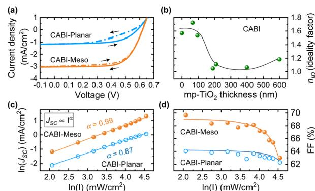
Fig. 3 (a)  $J$ - $V$  curves (reverse and forward bias scans) of the CABI-Meso and CABI-Planar champion cells. (b) Variation of the slope of  $V_{OC}$ -suns (*i.e.*, ideality factor) with the mp-TiO<sub>2</sub> layer thickness. (c) Log-log plot of  $J_{SC}$  versus 1-sun intensity for the devices. (d) FF variation with 1-sun intensity.
