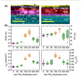
Fig. 2 (a) Cross-sectional SEM images of CABI-Meso (left) and CABI-Planar (right) photovoltaic cells. (b) Statistical distributions of the photovoltaic parameters of CABI devices as a function of mp-TiO<sub>2</sub> layer thickness, under 1-sun illumination.
