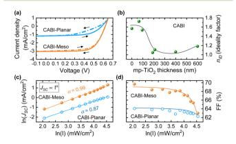
Fig. 3 (a) J-V curves (reverse and forward bias scans) of the CABI-Meso and CABI-Planar champion cells. (b) Variation of the slope of  $V_{\rm OC}$ -suns (i.e., ideality factor) with the mp-TiO<sub>2</sub> layer thickness. (c) Log-log plot of  $J_{SC}$  versus 1-sun intensity for the devices. (d) FF variation with 1-sun intensity.
