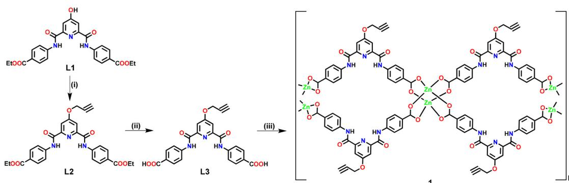
Scheme 1 Preparative route for the synthesis of Zn(II)-MOF **1**. Reaction conditions: (i) propargyl bromide, K<sub>2</sub>CO<sub>3</sub>; (ii) OH<sup>-</sup>; (iii) Zn(OAc)<sub>2</sub>.
