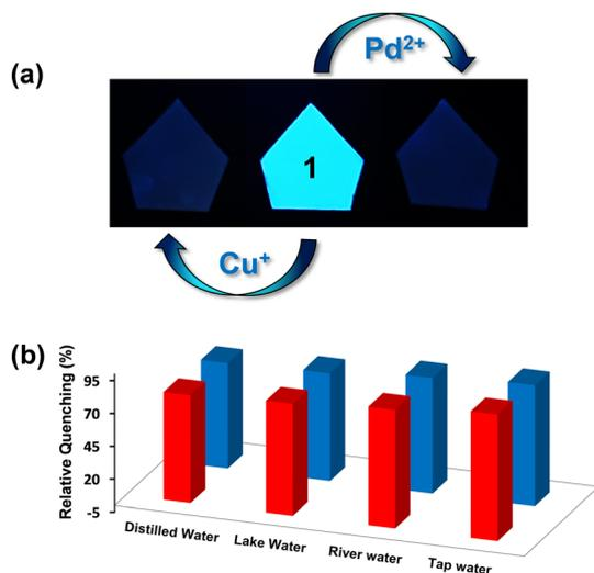
Fig. 7 (a) MOF-coated paper strips in the absence and presence of  $\text{Cu}^+$  and  $\text{Pd}^{2+}$  ions under UV light (365 nm) and (b) quenching efficiency of **1** for the  $\text{Cu}^+$  ion (28  $\mu\text{M}$ , red pillars) and  $\text{Pd}^{2+}$  ion (32  $\mu\text{M}$ , blue pillars) in various water samples (distilled water, lake water, river water, tap water).
