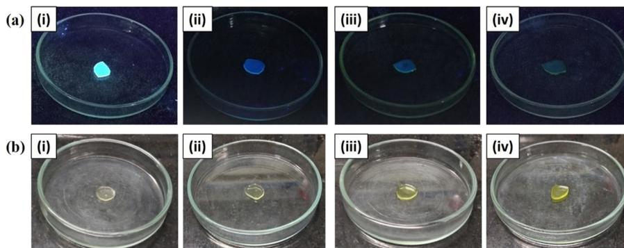
Fig. 12 Sensing response photographs of SAPAL-PY incorporated chitosan films with PA at concentrations of (i) 0 M, (ii)  $10^{-2}$  M, (iii)  $10^{-5}$  M, (iv)  $10^{-9}$  M under (a) UV lamp-365 nm and (b) visible light.
