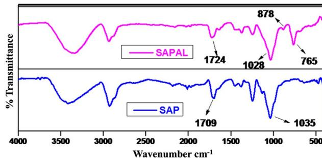
Fig. 5 FTIR spectra of SAP and SAPAL.
