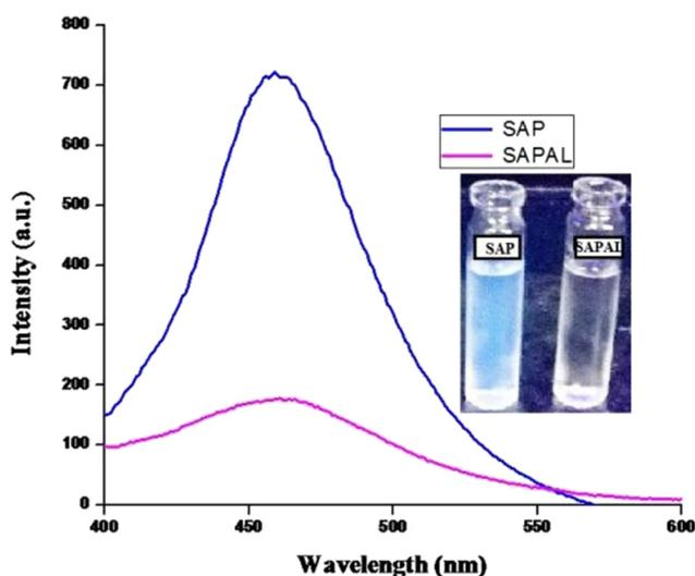
Fig. 4 Fluorescence emission spectra of SAP and SAPAL.
