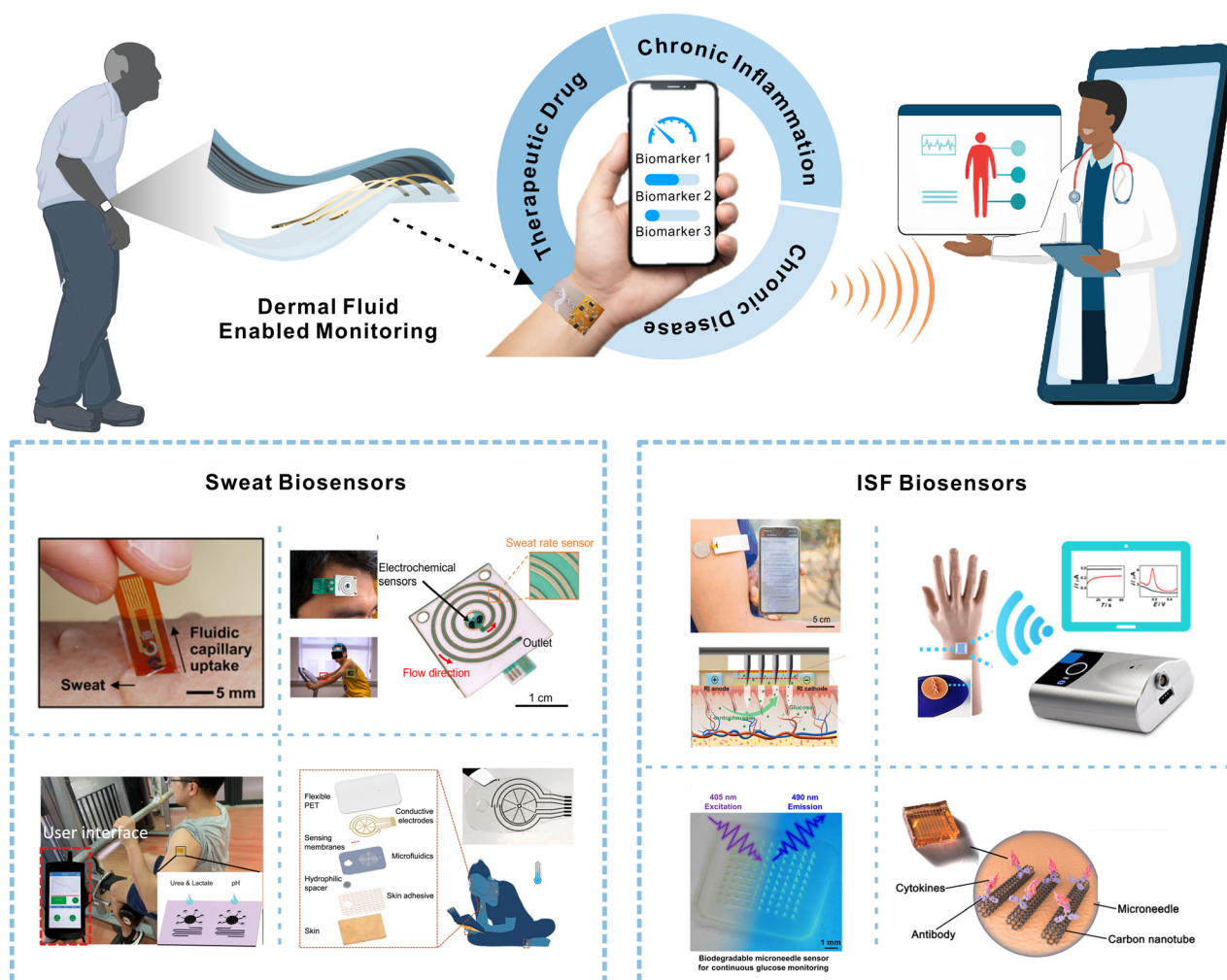
Fig. 1 Schematic depicting wearable dermal fluid-enabled biomarker detection for remote and non-invasive chronic disease, chronic inflammation, and therapeutic drug monitoring in ambulatory settings (top). The bottom illustration shows recently developed sweat and ISF biosensors for non-invasive analyte monitoring. Reprinted with permission from Lee et al. 15 Copyright© 2017 AAAS. Reprinted with permission from Nyein et al. 16 Copyright© 2021 Springer Nature. Reprinted with permission from Nyein et al. 17 Copyright© 2019 AAAS. Reprinted with permission from He et al. 18 Copyright© 2022 Springer Nature. Reprinted with permission from Cheng et al. 19 Copyright© 2022 Elsevier. Reprinted with permission from Goud et al. 20 Copyright© 2019 American Chemical Society. Reprinted with permission from Sang et al. 21 Copyright© 2023 AAAS. Reprinted with permission from Xu et al. 22 Copyright© 2023 Wiley-VCH GmbH.
