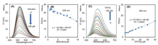
Fig. 4 (A) Change in fluorescence spectrum of THYQ-HSA (10:200) with increasing the concentration of bilirubin; (B) linear plot showing the decrease in fluorescence intensity at 555 nm with [bilirubin]; (C) change in fluorescence spectrum of BR-HSA (20:200) complex with [THYQ]; (D) linear plot showing the increase in fluorescence intensity at 555 nm with [THYQ].
