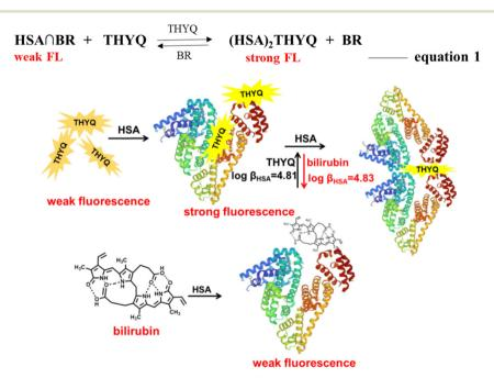
Scheme 2 Schematic presentation of the reversible displacement of THYQ by bilirubin and vice versa from its respective complex with HSAs.
