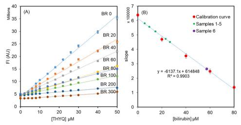
Fig. 5 (A) Titration of solutions of HSA (500  $\mu$ M) + bilirubin (0–300  $\mu$ M) with the probe THYQ; (B) linear relationship between the slopes and [bilirubin].
