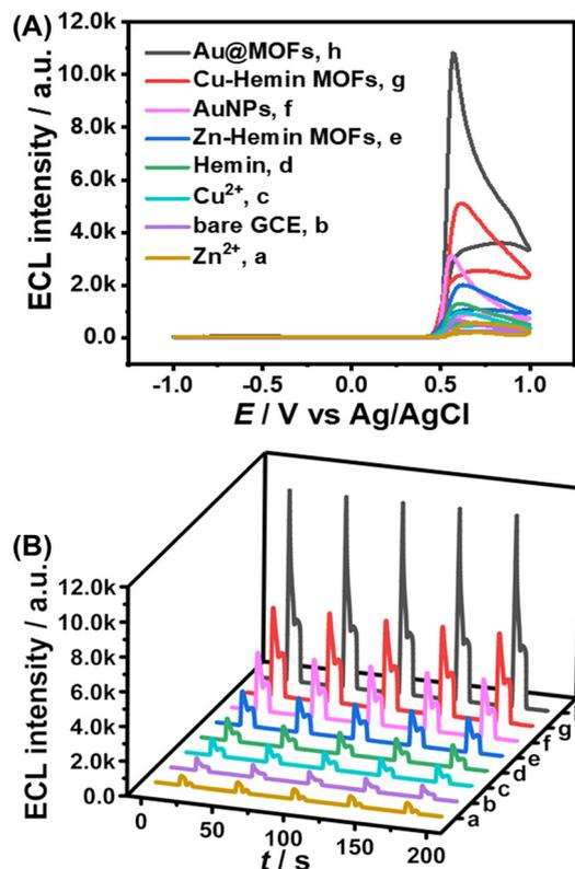
Fig. 2 ECL intensity-potential curve (A) and ECL intensity-time curve (B) of the modified electrodes. (a)  $\text{Zn}^{2+}$ /GCE, (b) bare GCE, (c)  $\text{Cu}^{2+}$ /GCE, (d) hemin/GCE, (e) Zn-hemin MOFs/GCE, (f) AuNPs/GCE, (g) Cu-hemin MOFs/GCE, and (h) Au@MOFs/GCE. All the experiments were conducted in 0.1 M PBS (pH = 7.4) containing 100  $\mu\text{M}$  luminol and 10 mM  $\text{H}_2\text{O}_2$ . Scan rate:  $0.1\text{ V s}^{-1}$ . Scan potential:  $-1.0$  to  $+1.0\text{ V}$ . PMT = 600 V.
