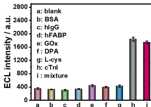
Fig. 5 Selectivity of the ESCL sensor for the detection of cTnI. cTnI concentration: 0.10 ng mL<sup>-1</sup>. Interference concentration: 1.0 ng mL<sup>-1</sup>. All the experiments were conducted in 0.1 M PBS (pH = 7.4) containing 100 μM luminol and 10 mM H<sub>2</sub>O<sub>2</sub>. a–i are the various possible interferences. Scan rate: 0.1 V s<sup>-1</sup>. Scan potential: -1.0 to +1.0 V. PMT = 600 V.
