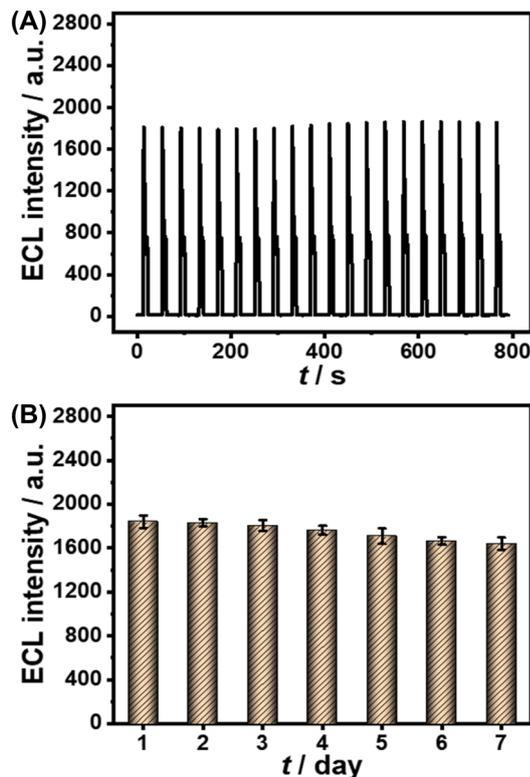
**Fig. 6** (A) ECL intensity–time curve of the ESCL immunosensor based on continuous CV scanning. (B) The inter-day stability of the ESCL sensor. All the experiments were conducted in 0.1 M PBS (pH = 7.4) containing 100  $\mu$ M luminol and 10 mM  $\text{H}_2\text{O}_2$ . cTnI concentration: 0.10 ng  $\text{mL}^{-1}$ . Scan rate: 0.1  $\text{V s}^{-1}$ . Scan potential:  $-1.0$  to  $+1.0$  V. PMT = 600 V.
