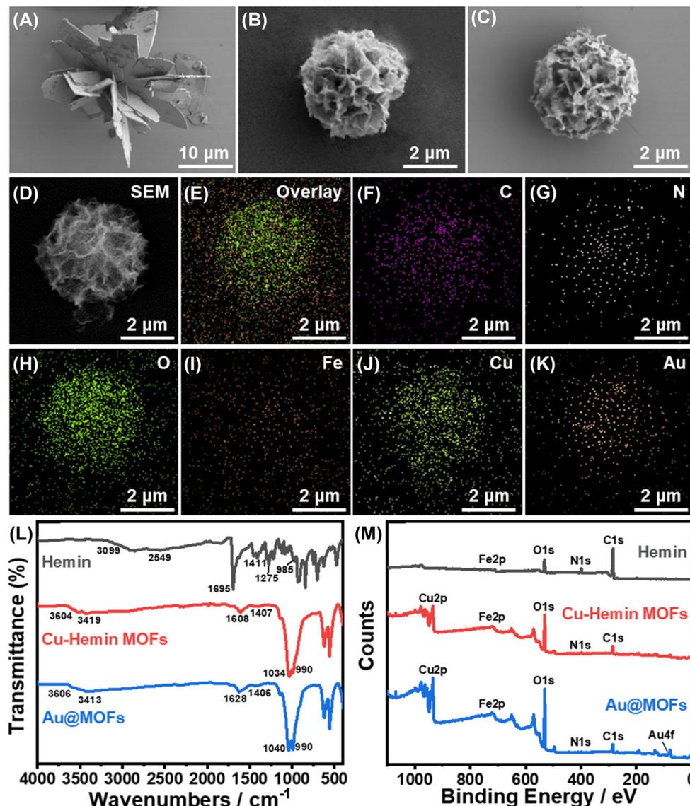
**Fig. 1** SEM images of Zn-hemin MOFs (A), Cu-hemin MOFs (B) and Au@MOFs (C). (D–K) SEM image of Au@MOFs and the corresponding element distribution. (L) FT-IR spectra of hemin (black curve), Cu-hemin MOFs (red curve), and Au@MOFs (blue curve). (M) XPS spectra of hemin (black curve), Cu-hemin MOFs (red curve), and Au@MOFs (blue curve).
