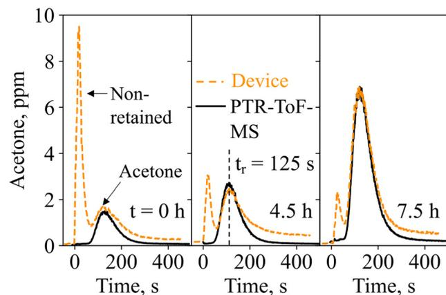
**Fig. 4** Acetone concentrations as recorded by the device (dashed line) and PTR-ToF-MS (solid line) for three exhalations of volunteer #1 at  $t = 0$  h (at 8:00), 4.5 h and 7.5 h of the ketogenic diet. The acetone retention time ( $t_r$ ) is indicated with a dashed line.
