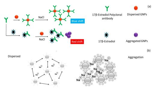
Fig. 8 Development of colorimetric approach for the detection of estriol. a) Antibody-based colorimetric detection of 17-β-estriol using AuNPs under appropriate salt condition and b) nature of AuNPs in the presence of a high salt concentration. Reproduced from ref. 85 with permission from [Elsevier], Copyright [2020].
