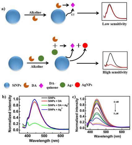
Fig. 11 a) Schematic representation for the detection of DA using SiNPs, b) fluorescence spectra of SiNPs and SiNPs in the presence of DA, DA<sup>+</sup> and Ag<sup>+</sup> and c) change in fluorescence intensity with an increase in the concentration of DA (0 nM to 5  $\mu$ M). Reproduced from ref. 96 with permission from [Elsevier], Copyright [2018].
