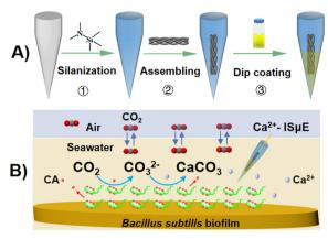
Fig. 1 (A) Schematic diagram of the preparation process of CNT fiber/ Ca<sup>2+</sup>-ISμE. (B) Schematic diagram of monitoring the dynamic changes in  $Ca^{2+}$  concentration above the biofilm using  $Ca^{2+}$ -IS $\mu E$ .
