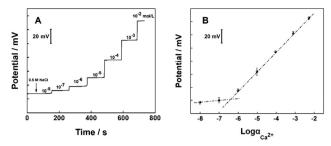
Fig. 3 (A) Potentiometric responses of the CNT fiber/Ca<sup>2+</sup>-IS $\mu$ E in 0.5 M NaCl. (B) Calibration curve of the CNT fiber/Ca<sup>2+</sup>-IS $\mu$ E. Error bars represent the standard deviation for three measurements.
