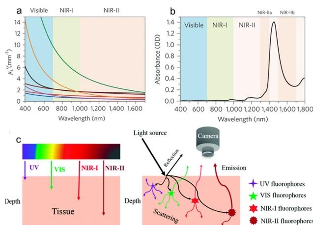
**Fig. 1** a) The scattering coefficients of different wavelengths covering the visible, NIR-I and NIR-II windows. b) Absorption spectrum of water in the spectral range of 400–1800 nm. c) Schematic illustration of tissue penetration depth and light–tissue interaction of different wavelengths. Reproduced with permission Copyright©2018, The Royal Society of Chemistry.<sup>15</sup>
