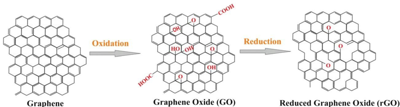
Fig. 2 General structure of graphene, carboxyl-functionalized graphene oxide and reduced graphene oxide nanomaterials (with permission from Springer, copyright [2018]<sup>50</sup>).
