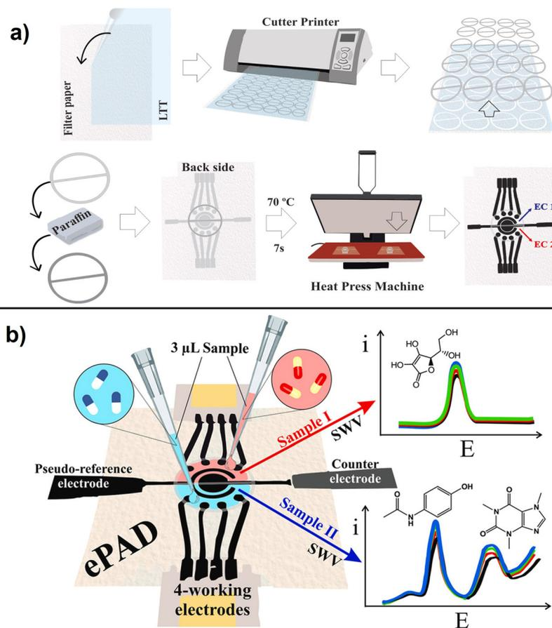
**Fig. 6** Schematic representation of multiplexed (4 WE) ePAD fabrication showing a), steps in the fabrication process using a cutter printer involving wax barrier production and b), illustration of the integrated ePAD for multi-analyte detection using SWV (with permission of Elsevier, copyright [2019]<sup>85</sup>).
