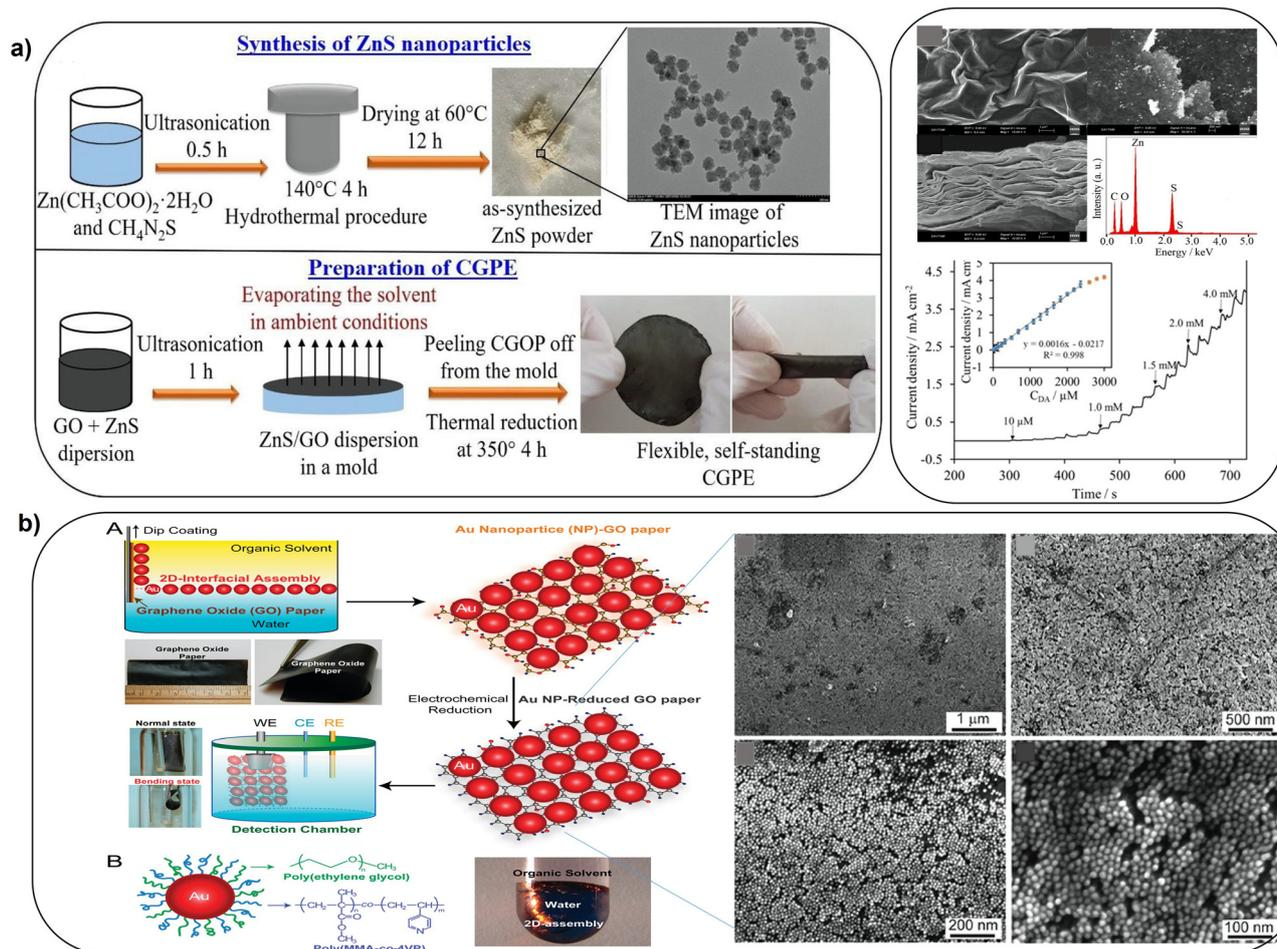
**Fig. 7** Schematic illustration of: a), synthesis of ZnS NPs and deposition of GO and ZnO as a flexible standalone CGPE sensor (with permission from Wiley, copyright [2021]<sup>87</sup>) and b), the fabrication of freestanding hybrid electrodes from 2D-assembly of AuNPs and GO-modified paper, with SEM images of 2D-assembly of AuNPs coated on GO paper at different magnifications (with permission from ACS, copyright [2012]<sup>88</sup>).
