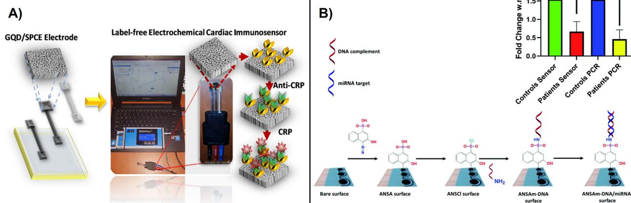
**Fig. 10** A) Fabrication of SPCE immunosensor and portable electrochemical detection set-up for detection of C-reactive protein (CRP) (with permission from ACS, copyright [2021]<sup>116</sup>), and B) modification of SPE with diazo-sulfonamide modified and DNA for detection of microRNA expression in samples from diabetic kidney disease patients, as compared to controls (inset shows comparative results between sensor data and RT-qPCR) (with permission from RSC, copyright [2021]<sup>118</sup>).
