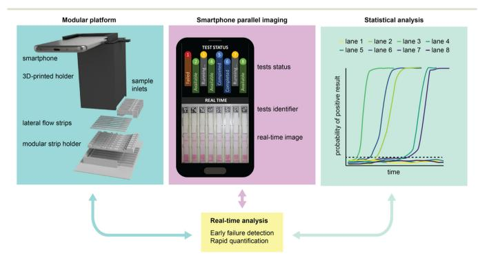
Fig. 1 Overview of the LFIA processing platform, combining a 3D-printed modular platform, smartphone-assisted imaging, and advanced statistical analysis to monitor and read LFIA tests in real time.
