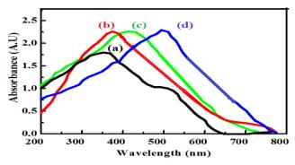
Fig. 1 UV-vis absorbance spectra of (a) Co<sub>3</sub>O<sub>4</sub> NPs, (b), ZnO NPs, (c) ZnO/Co<sub>3</sub>O<sub>4</sub> nanocomposite and (d) ZnO/Co<sub>3</sub>O<sub>4</sub>/rGO nanocomposite.
