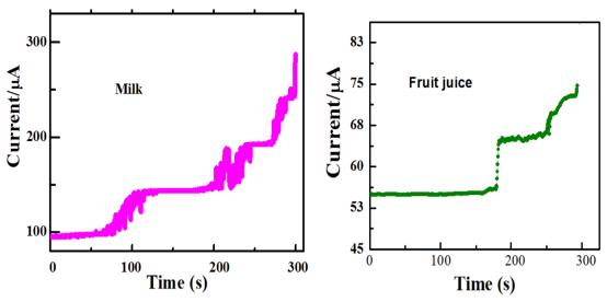
Fig. 14 Amperometric responses of ZnO/Co<sub>3</sub>O<sub>4</sub>/rGO/GCE towards two different real samples (milk and fruit juice) in 0.1 M NaOH at an applied potential of 0.55 V.
