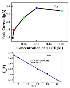
Fig. 8 (A) The plot of anodic current of ZnO/Co<sub>3</sub>O<sub>4</sub>/GCE versus different concentrations of NaOH (0.005 M up to 0.2 M) upon the addition of 2 mM glucose at a scan rate of 50 mV s<sup>-1</sup>. (B) The plot of anode potential ( $E_{pa}$ ) vs. pH values NaOH.
