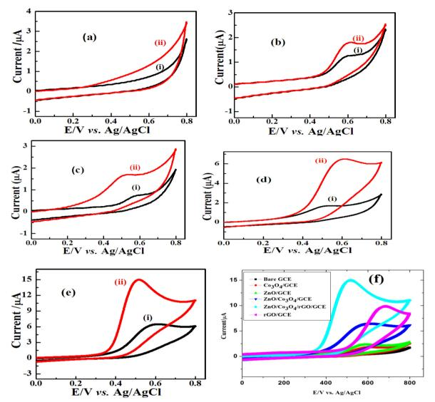
Fig. 5 CVs of (a) bare GCE, (b) Co<sub>3</sub>O<sub>4</sub>/GCE, (c) ZnO/GCE, (d) ZnO/Co<sub>3</sub>O<sub>4</sub>/GCE, (e) ZnO/Co<sub>3</sub>O<sub>4</sub>/rGO/GCE in the absence (i), presence (ii) of 2 mM glucose and (f) electrodes under study in the presence of 2 mM glucose in 0.1 M NaOH at a 50 mV s $^{-1}$  scan rate.
