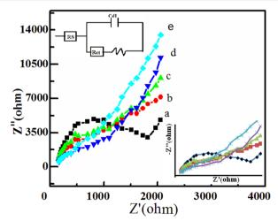
Fig. 7 EIS measurement of bare electrode (a), Co<sub>3</sub>O<sub>4</sub>/GCE (b), ZnO/ GCE (c), ZnO/Co<sub>3</sub>O<sub>4</sub>/GCE (d) and ZnO/Co<sub>3</sub>O<sub>4</sub>/rGO/GCE (e) in 0.1 M NaOH solution containing 2 mM glucose. The inset circuit is the equivalent circuit used for the EIS data analysis.
