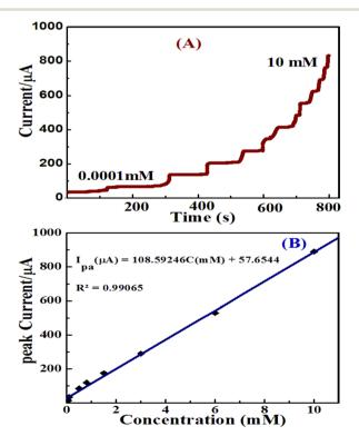
Fig. 10 (A) A typical amperometric i-t curve of ZnO/Co<sub>3</sub>O<sub>4</sub>/rGO electrode to successive addition of glucose solution into a stirred system of 0.1 M NaOH (pH 13.0) at +0.55 V. Rotating speed 3000 rpm. (B) Linear calibration plot of the corresponding current *versus* the glucose concentration.
