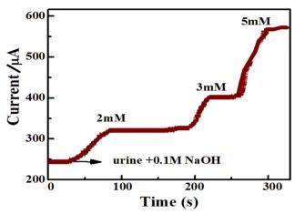
Fig. 13 Amperometric i-t response of ZnO/Co<sub>3</sub>O<sub>4</sub>/rGO/GCE for successful injection of the standard glucose solution (2, 3, and 5 mM) at an applied potential of 0.55 V, with a rotation speed of 1000 rpm.
