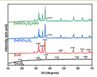
Fig. 3 XRD patterns of, Co<sub>3</sub>O<sub>4</sub> NPs, ZnO NPs, ZnO/Co<sub>3</sub>O<sub>4</sub> and ZnO/ Co<sub>3</sub>O<sub>4</sub>/rGO nanocomposites.
