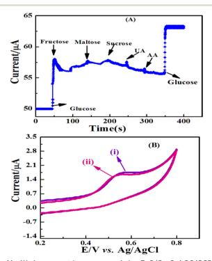
Fig. 11 (A) Amperometric response of the ZnO/Co<sub>3</sub>O<sub>4</sub>/rGO/GCE in 0.1 M NaOH (pH 13) upon the successive addition of glucose (1 mM), fructose (0.1 mM), maltose (0.1 mM), sucrose (0.1 mM), UA (0.1 mM), AA (0.1 mM), and 1 mM glucose, respectively, (B) CVs of a ZnO/Co<sub>3</sub>O<sub>4</sub>/rGO/GCE containing 1 mM glucose and 0.1 M NaOH solution (curve i) and in the presence of 0.05 M NaCl (curve ii) at a scan rate of 50 mV s<sup>-1</sup>.
