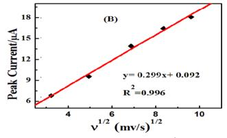
Fig. 6 (A) Effect of the scan rate (10-100 mV s<sup>-1</sup>) on the cyclic voltammogram ZnO/Co<sub>3</sub>O<sub>4</sub>/rGO in the presence of 0.1 M NaOH and 2 mM glucose. (B) The plot of current against the square of the scan rate  $(v^{1/2}).$
