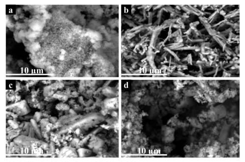
Fig. 4 SEM images of a) ZnO, b) Co<sub>3</sub>O<sub>4</sub>, c) ZnO/Co<sub>3</sub>O<sub>4</sub>, and d) ZnO/Co<sub>3</sub>O<sub>4</sub>/rGO
