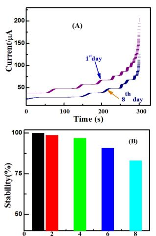
Fig. 12 (A) The first-day and eighth-day amperometric responses of the ZnO/Co<sub>3</sub>O<sub>4</sub>/rGO/GCE in 0.1 M NaOH upon the successive addition of 2 mM glucose at 0.55 V, (B) the percent stability of the ZnO/Co<sub>3</sub>O<sub>4</sub>/ rGO nanocomposite sensor for eight days.
