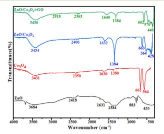
Fig. 2 FTIR spectrum of ZnO NPs, Co<sub>3</sub>O<sub>4</sub> NPS, ZnO/Co<sub>3</sub>O<sub>4</sub> nanocomposite, and ZnO/Co<sub>3</sub>O<sub>4</sub>/rGO nanocomposite.
