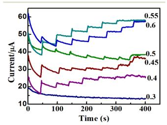
Fig. 9 Amperometric i-t graphs of ZnO/Co<sub>3</sub>O<sub>4</sub>/rGO/GCE to the successive injections of 2 mM glucose at different applied potentials from 0.3 V up to 0.6 V.
