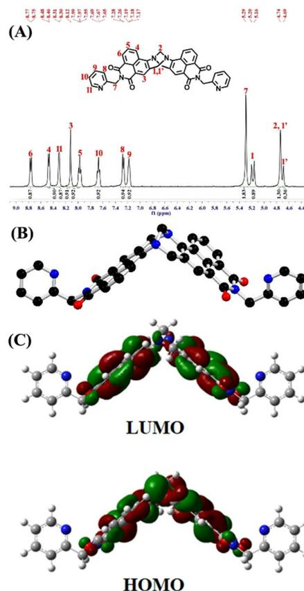
**Fig. 1** (A)  $^1\text{H}$  NMR spectrum of **TBNap** (400 MHz,  $\text{DMSO}-d_6$ ) with peak assignment. (B) Energy-minimized structure of **TBNap** (colour code: black C, red O, and blue N). Hydrogen atoms are omitted for clarity. (C) The frontier molecular orbitals of **TBNap**.
