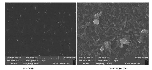
Fig. 8 SEM images of probe Me-INDP and probe with CN<sup>-</sup> concentration.
