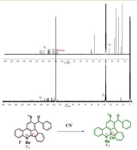
Fig. 5 <sup>13</sup>C NMR spectrum for reactant Me-INDP (bottom) and product after addition with CN<sup>-</sup> (above) (in d<sub>6</sub>-DMSO).
