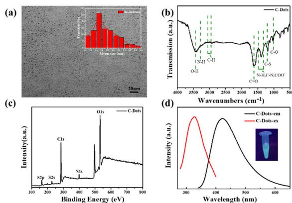
**Fig. 1** (a) TEM image of C-dots (inset: size distribution of the C-dots). (b) FT-IR spectrum of C-dots. (c) Full scan XPS survey spectrum of C-dots. (d) Fluorescence spectra of C-dots (excitation wavelength: 320 nm, emission wavelength: 420 nm, inset: C-dot solution under UV light at 365 nm).
