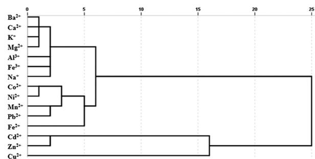
Fig. 4 Hierarchical cluster analysis (HCA) of the sensor array data for various metal ions.
