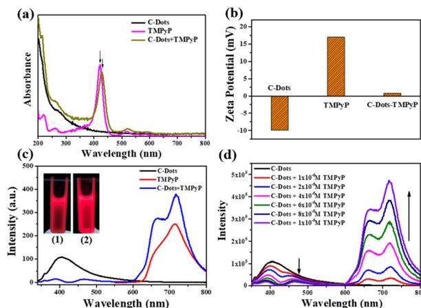
**Fig. 2** (a) UV-vis spectra of C-dots, TMPyP and C-dot-TMPyP. (b) Zeta potentials of C-dots, TMPyP and C-dot-TMPyP. (c) Fluorescence emission spectra of C-dots, TMPyP and C-dot-TMPyP (the excitation wavelengths were 320 nm, 420 nm and 320 nm, inset: images of TMPyP (1) and C-dot-TMPyP (2) under UV light at 365 nm). (d) Fluorescence spectra of C-dots in the presence of increasing TMPyP concentrations (0–10  $\mu\text{M}$ ) (the excitation wavelength was 320 nm).
