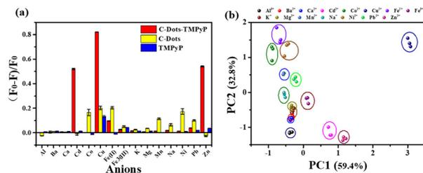
Fig. 3 (a) Fluorescence responses of the three sensors after adding various ions.  $F$  and  $F_0$  present the fluorescence responses of the sensors with and without metal ions. The error bar height represents one standard deviation of the three replicate. (b) Plot of analytes derived from the multivariate data by PCA.
