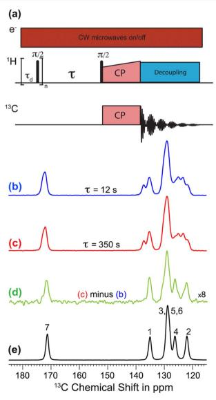
Fig. 1 (a)  $^{1}H^{-13}C$  CPMAS saturation–recovery pulse sequence used to record solid-state  $^{13}C$  NMR spectra for different polarization times ( $\tau$ ). (b and c) DNP-enhanced solid-state  $^{13}C$  NMR spectra of powdered m-ABA recorded at 110 K with (b)  $\tau = 12$  s and (c)  $\tau = 350$  s. (d) Difference spectrum. (e) Solid-state  $^{13}C$  NMR spectrum recorded at 110 K for a sample of pure Form III m-ABA. Reproduced with permission from ref. 15.
