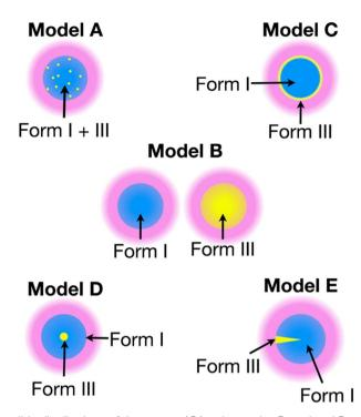
Fig. 2 Models A-E show different possible distributions of the two m-ABA polymorphs, Form I and Form III. The solution (pink) containing the polarizing agent is located on the surface of the particles. Numerical simulations of  $^1H$  spin diffusion suggested that model B best reproduced the DNP saturation recovery experiments. Reproduced with permission from ref. 15.
