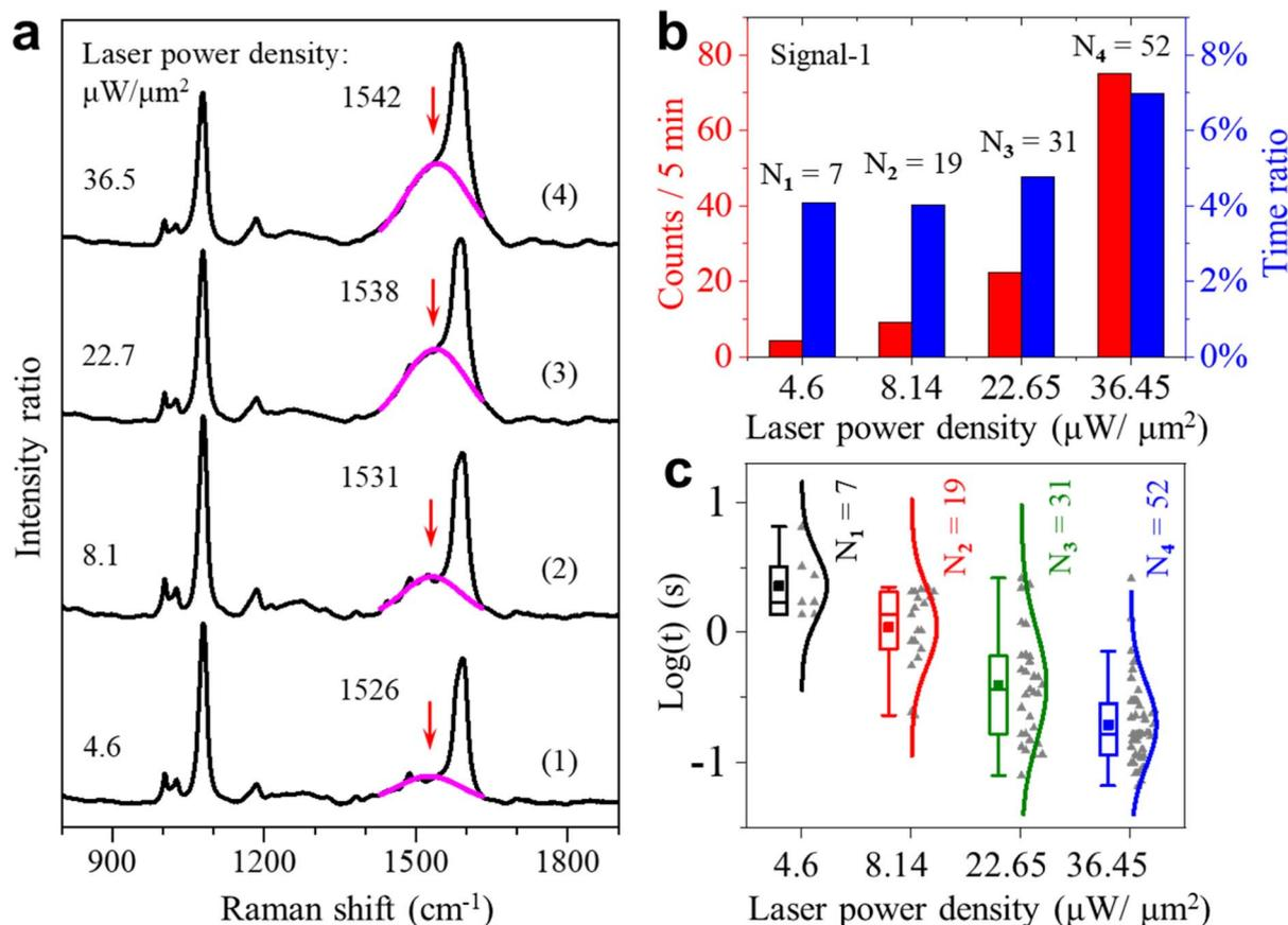
Fig. 3 (a) Four representative averaged SERS spectra under four different laser power densities. The pink lines are the Gaussian fits to the broad peaks near 1531  $\text{cm}^{-1}$ . (b) Appearance event counts (red) and total appearance time percentage (blue) for signal-1 under different laser power densities. (c) Lifetime of signal-1 on the logarithmic scale under four different laser power densities.
