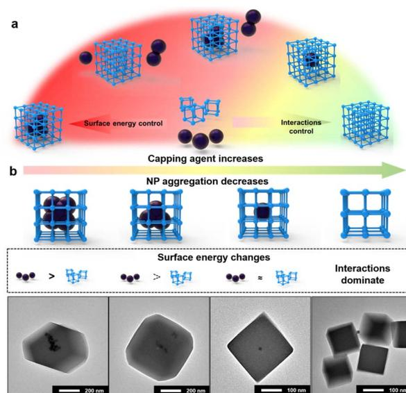
Fig. 3 (a) Summary of the mechanism of *de novo* NP encapsulation. (b) When the surface energy of metal NPs is greater than that of MOF-PNC, the addition of free end capping agents leads to a specific core-shell structure due to the fine-tuning of the surface energy difference.
