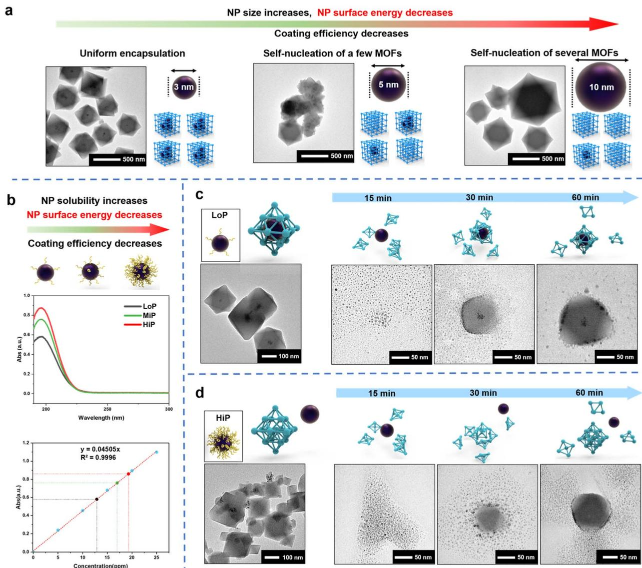
**Fig. 1** (a) With the increase in the size of Pt NPs, the coating efficiency decreases. (b) UV absorption of PVP on 3 nm LoP (black), 3 nm MiP (green) and 3 nm HiP (red). (c) TEM images of LoP@UiO-66 and time-dependent studies of the synthesis of LoP@UiO-66. (d) TEM images of HiP@UiO-66 and time-dependent studies of the synthesis stages of HiP@UiO-66. A high concentration of capping agents on Pt NPs leads to a decrease in the surface energy.
