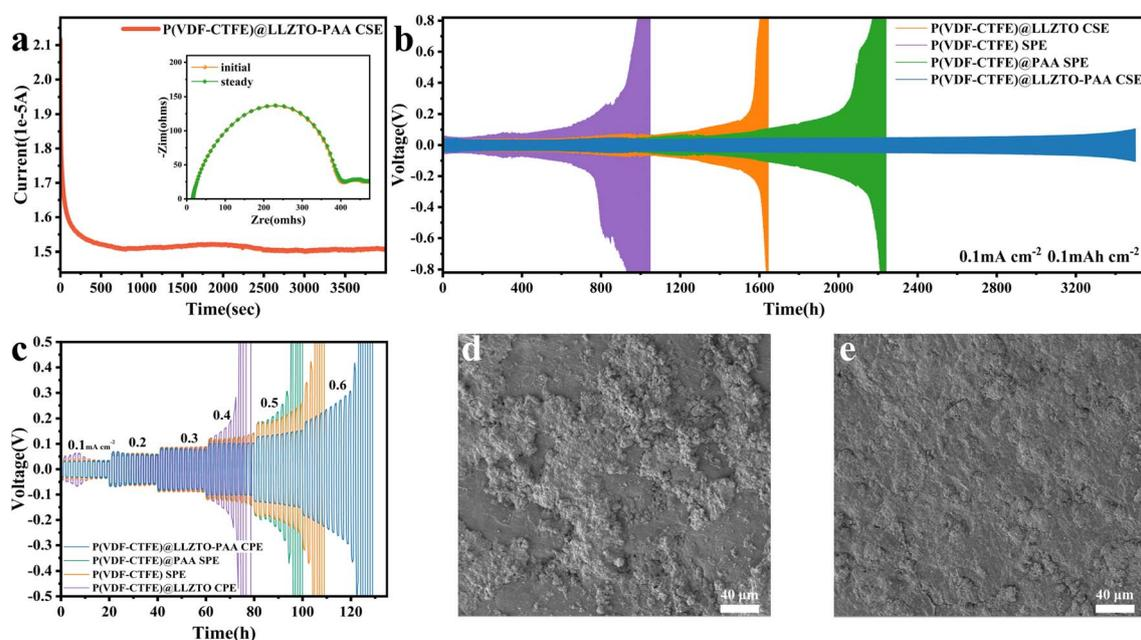
Fig. 5 (a) Chronoamperometry profile of the Li/Li symmetric cell for P(VDF-CTFE)@LLZTO-PAA CSE. The inset shows the EIS curves before and after polarization. (b) Cycling performance of Li||SSEs||Li cells plating/stripping. (c) The critical current density test of Li||SSEs||Li cells. The surface morphologies of lithium metal after 200 h: (d) Li||P(VDF-CTFE)@LLZTO CSE||Li and (e) Li||P(VDF-CTFE)@LLZTO-PAA CSE||Li.
